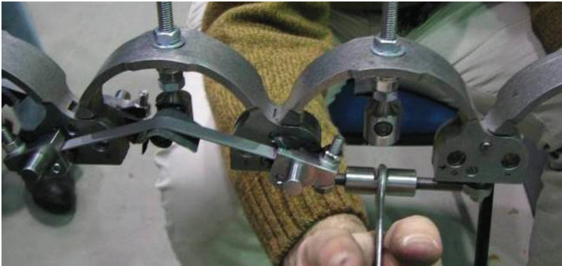
Figure 22: Assembly of the SMA ribbon to each titanium arc by means of the puller.
