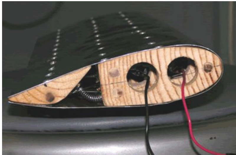
Figure 78: Wing section with deformable trailing edge actuated by SMA wires. [87]
