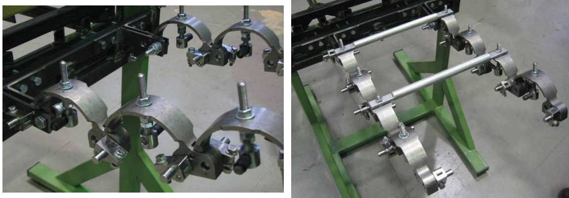
Figure 21: View of the two arc series (ribs), without SMA ribbons, attached to the support frame.
