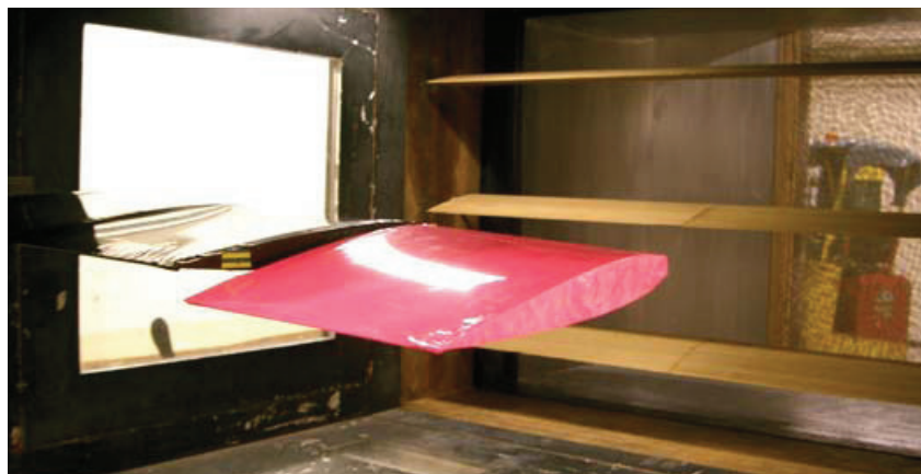
Figure 110: Load alleviation device using an all-moving wing tip. [120]
