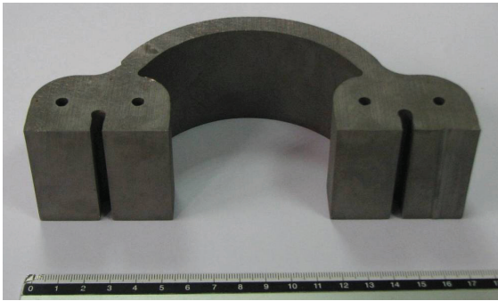
Figure 6. Arch manufacture: initial milling of the solid block of titanium.
