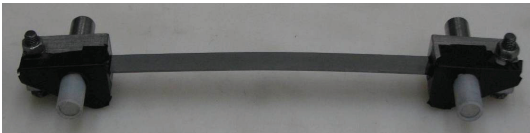
Figure 17. View of the unstrained SMA ribbon, secured to the clamps, both insulated.
