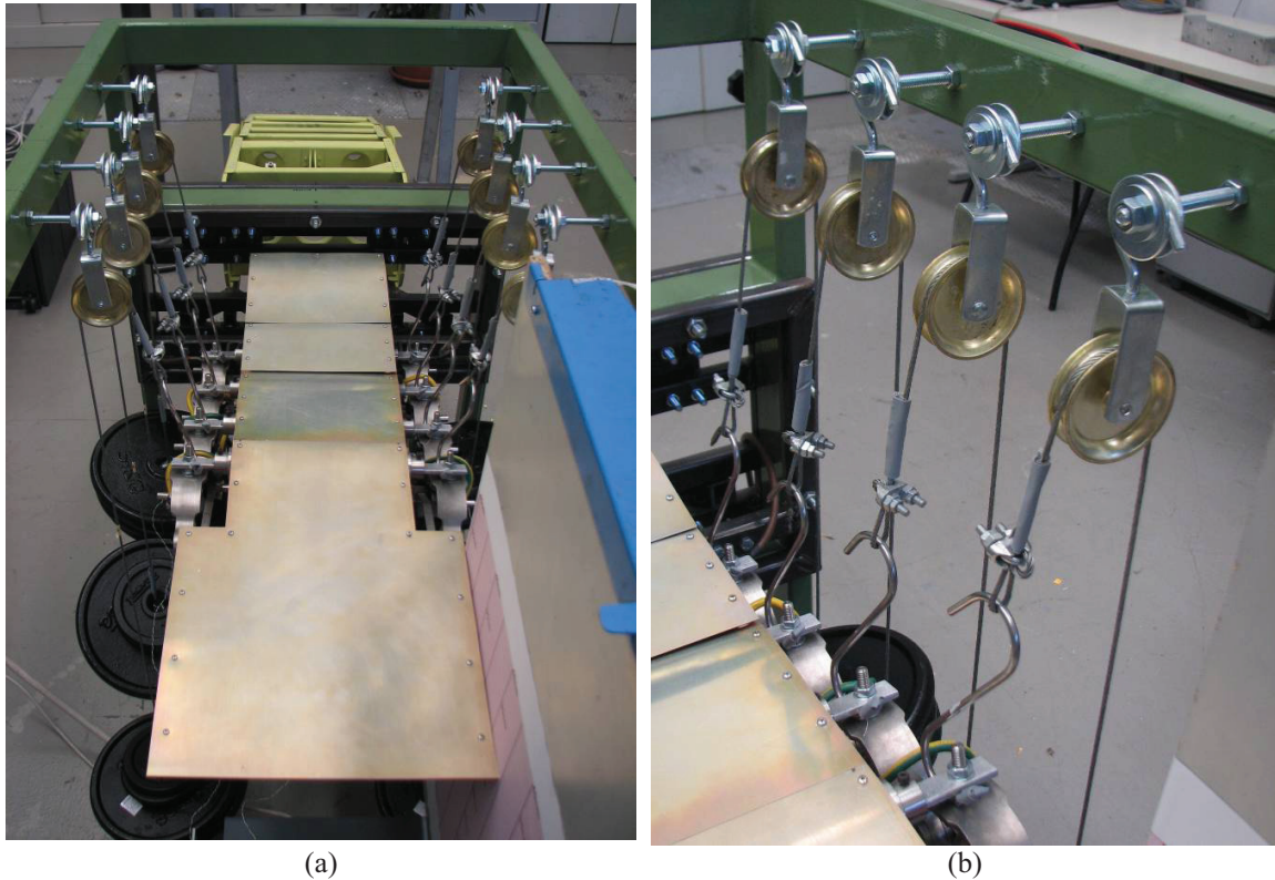
Figure 29: Details of the pulley, cables and weights system used to apply static loads to the flap prototype.
