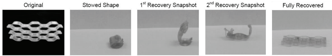
Figure 154: Veriflex® honeycomb structure self-recovering under an IR heat lamp. [208]
