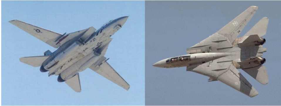
Figure 1: F-14 Tomcat: variable sweep mechanism in the extended (left) and retracted (right) position.
