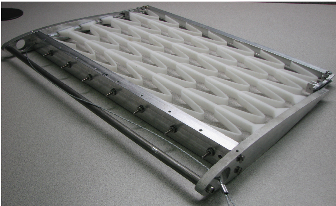
Figure 49: Almost complete assembly: details of the actuation wire and the accordion connection to the front spar.
