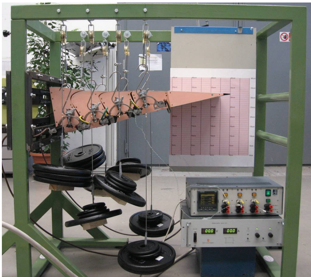
Figure 28: View of the full experimental setup for the test campaign in presence of static loads.
