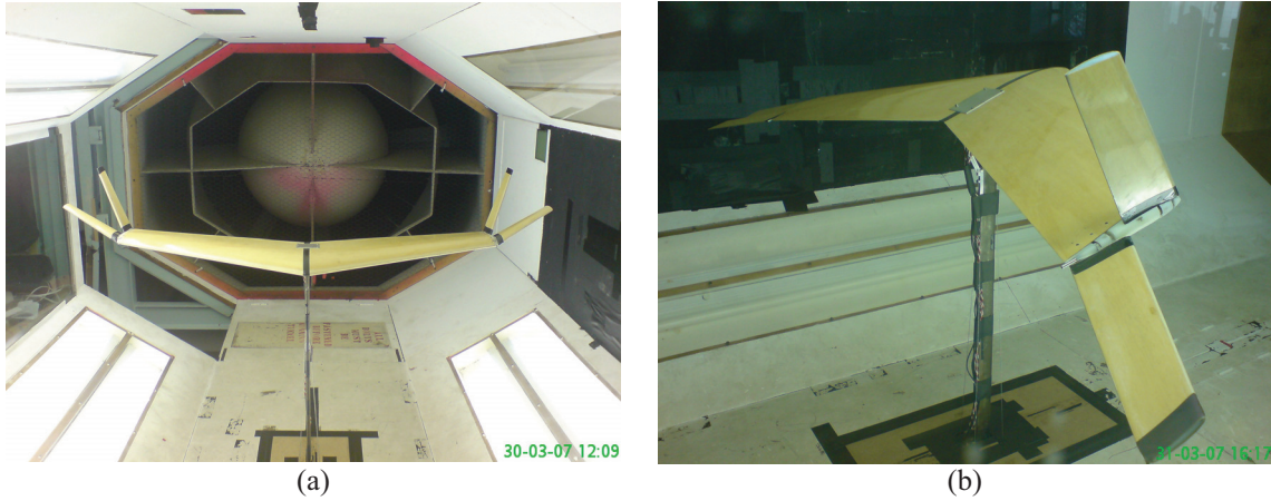
Figure 108: Experimental model as mounted in the wind-tunnel: (a) front and (b) rear view. [115]
