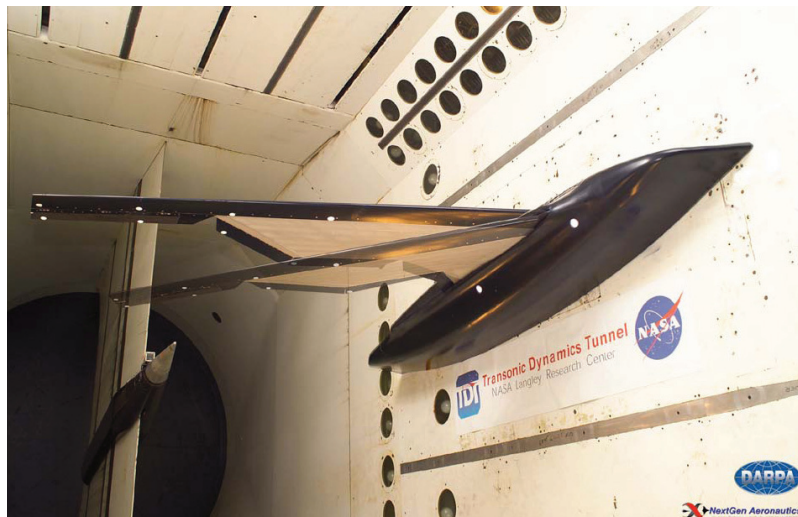
Figure 74: NextGen Aeronautics half MFX-1 wind tunnel tests. [43]
