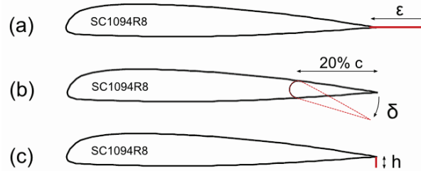
Figure 1: Trailing edge devices: (a) Static Extended Trailing Edge (SETE), (b) Trailing Edge Flap (TEF), and (c) Gurney Flap (GF).
