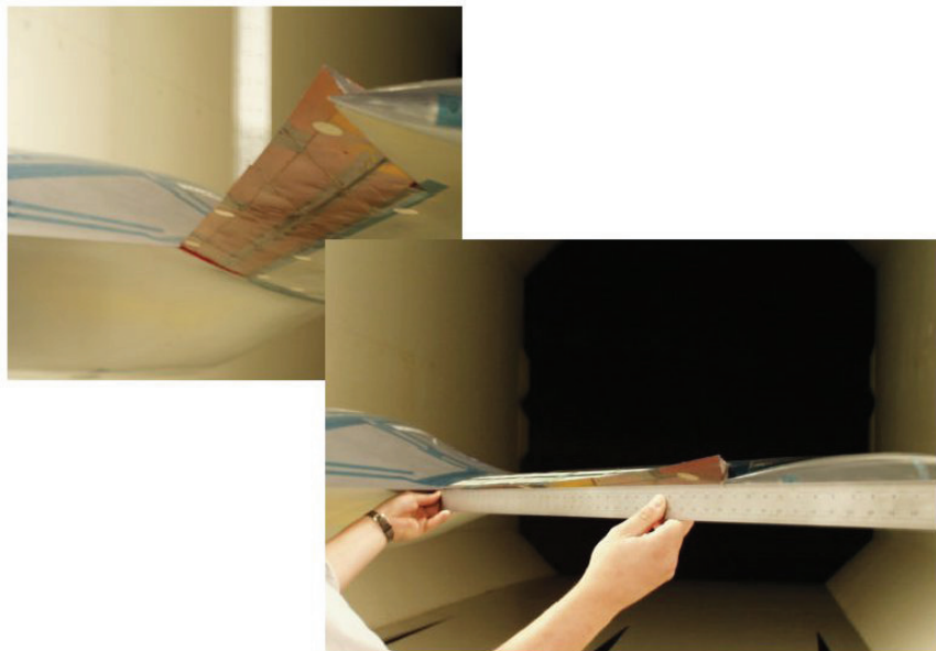
Figure 99: UCAV trailing edge deflection tests. [93, 94]
