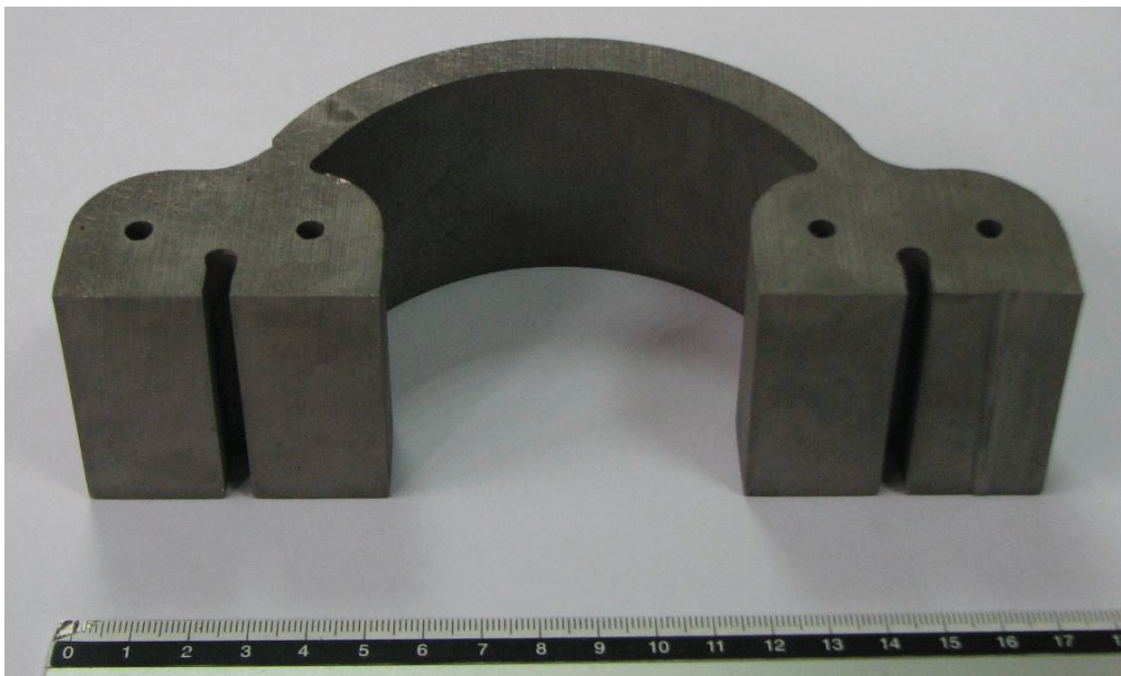
Figure 27. Arch manufacture: initial milling of the solid block of titanium.
