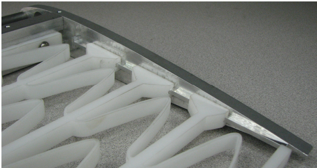
Figure 46: Airfoil and accordion assembly: details of the sliding guide.
