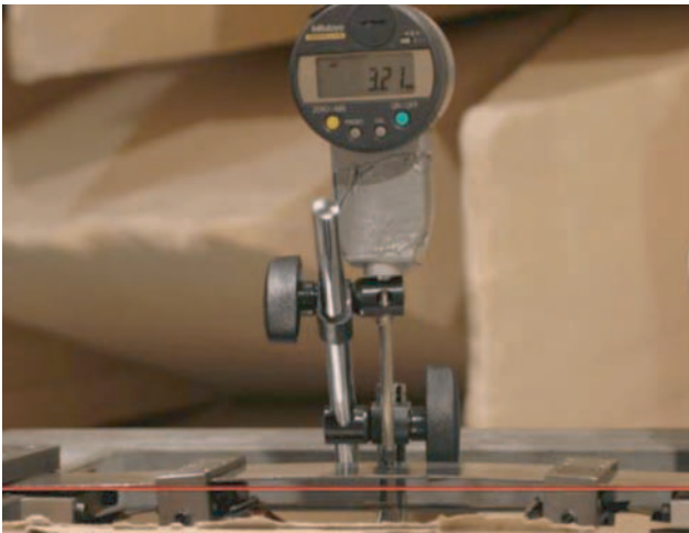
Figure 22. Bump profile for SMA ribbon with a 1.5% initial deformation: maximum bump height of 3.21 mm.
