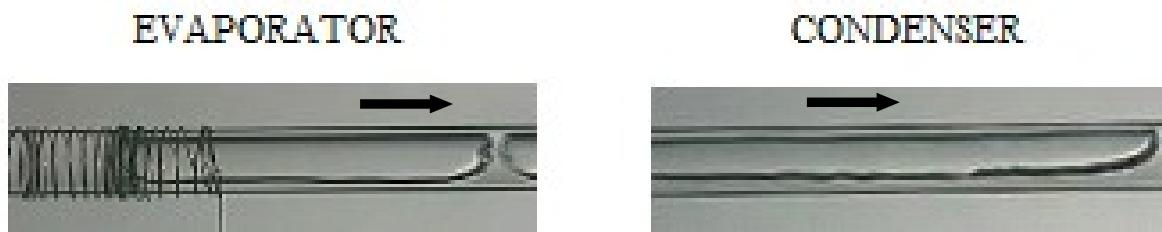
**Figure 4.15 - Slug boiling behaviour in self-rewetting fluid (horizontal configuration). Input power 18W.**
