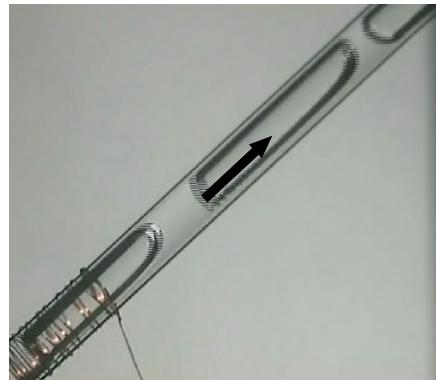
**Figure 4.12 - Slug boiling behaviour in water  $\alpha = 45^\circ$ . Input power 18W.**
