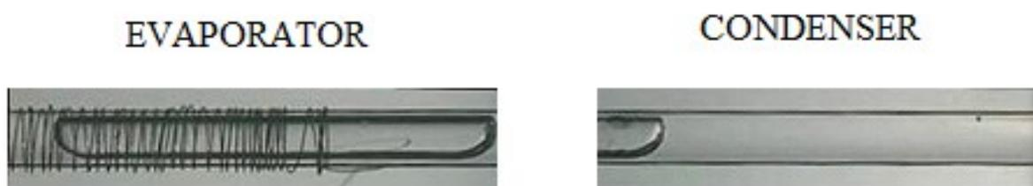
**Figure 4.14 - Dry-out behaviour in water (horizontal). Input power 18W.**
