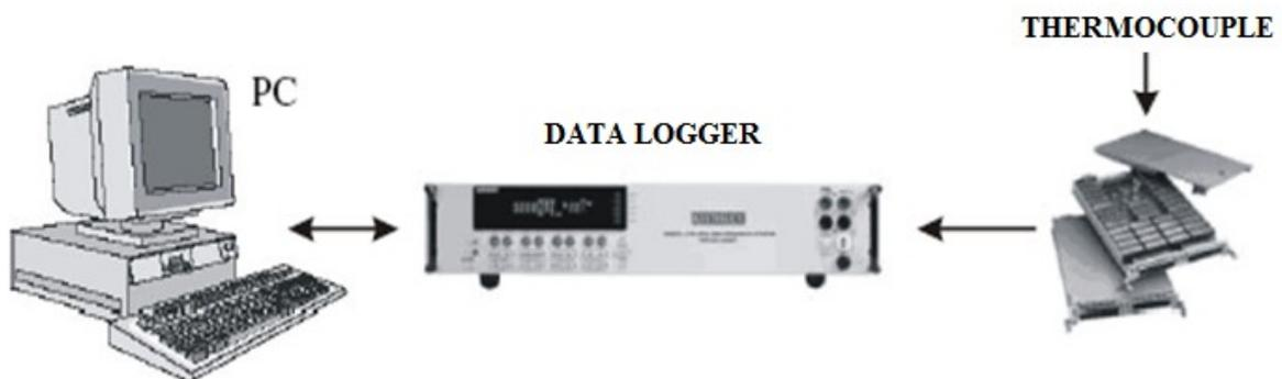
**Figure 4.2 – Data acquisition system.**
