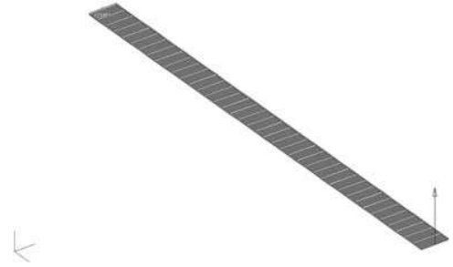
Figure 8. FE Model of the referred cantilever beam.
