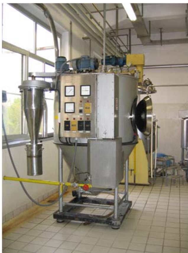
Fig. 7.1: Pilot plant: Spray dryer.
