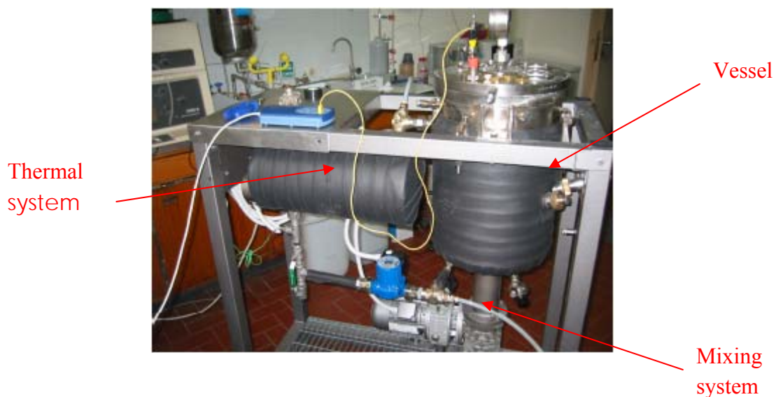
Fig. 5.2: Pilot plan: Fermenter.
