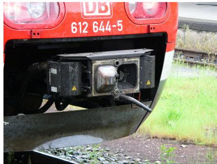
**Fig. 3.15 - Automatic coupler Scharfenberg [13].**
