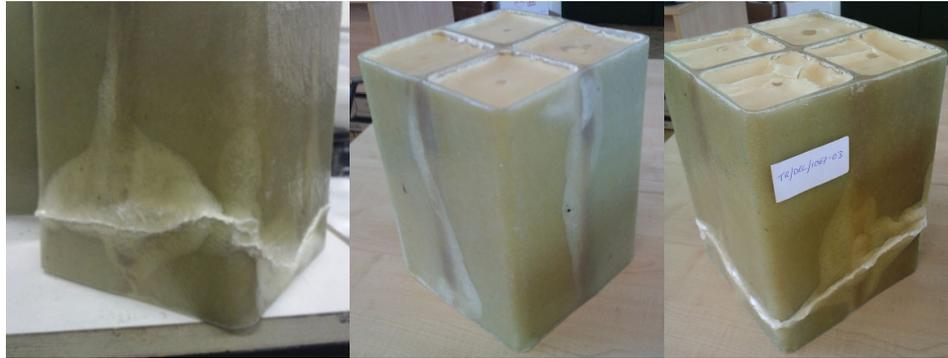
**Fig. 6.33 – Detail of the failure occurred during compression tests on the FRP and polyurethane foam specimens.**
