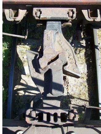
**Fig. 3.14 - Wilson system in the coupling configuration [13].**
