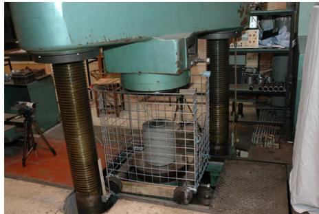
Fig. 4.2 – Test machine used for compression tests.
