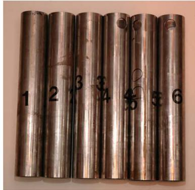
Fig. 4.1 – Mild steel samples for compression tests.
