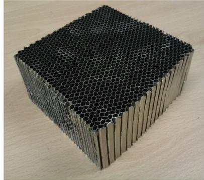
**Fig. 5.4 – Aluminium honeycomb block tested.**
