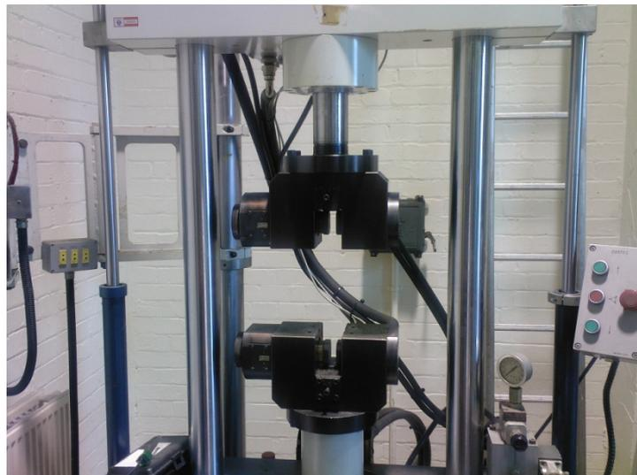
**Fig. 5.5 – DARTEC - Testing machine for static and dynamic test.**
