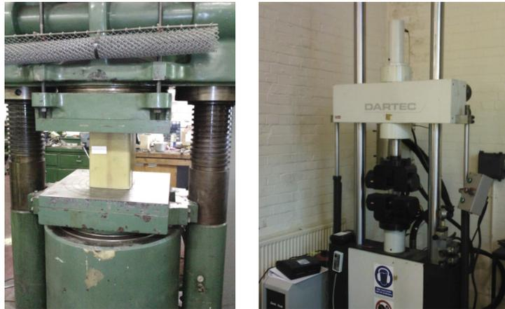
**Fig. 6.31 – (a) Avery-Denison compression loading machine, (b) DARTEC Universal Test Machine.**
