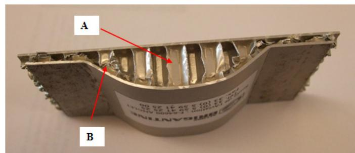
**Fig. 5.13 – Specimen configuration after test with non continuum support.**
