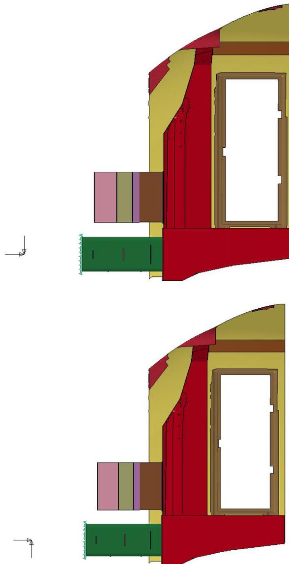
**Fig. 6.40 – Vertical load applied on the buffer level on a single node rigid constrained to the anticlimber – VS\_1 (a) and VS\_2 (b).**
