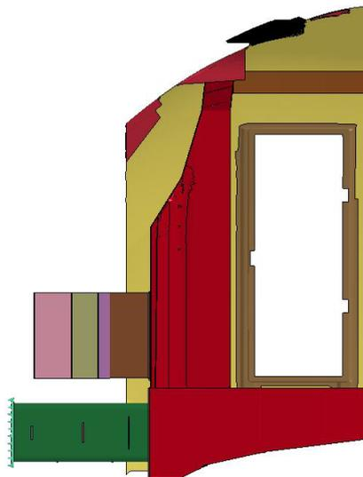
**Fig. 6.39 – Nodal Load applied at the level of the cant rail.**
