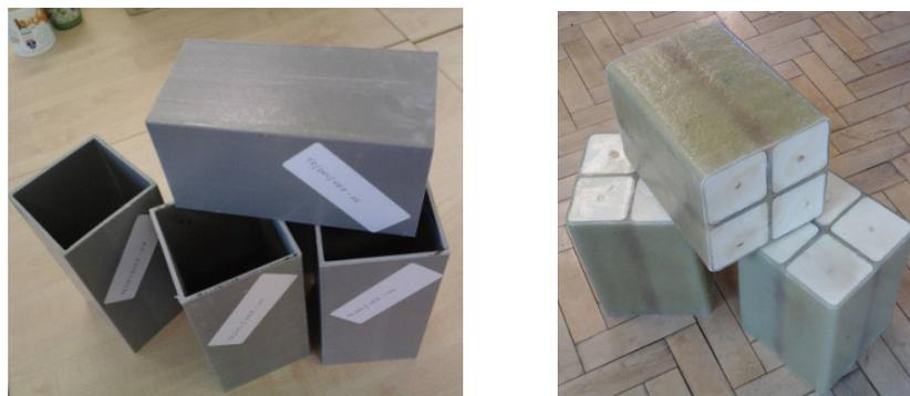
**Fig. 6.32 – (a) GRP tubes, (b) Specimens made by polyurethane foam and glass epoxy.**
