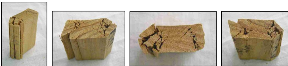
Figure 6.33. Compression tests perpendicular to grain on specimens type DF-C rad – Typical radial collapse mechanisms consisting in large transversal deformations.
