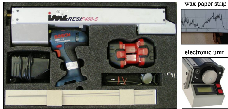
Figure 5.20. Resistographic tests – Testing apparatus: IMLRESI F400 device.
