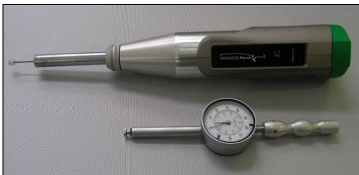
Figure 5.12. Sclerometric tests – Testing apparatus: Wood Pecker mechanical tests hammer.
