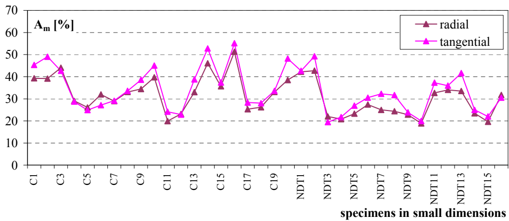
Figure 5.31. Resistographic tests – Experimental results of specimens type S_S -C and S_S -NDT: comparison between radial and tangential mean amplitude ( A_m ).
