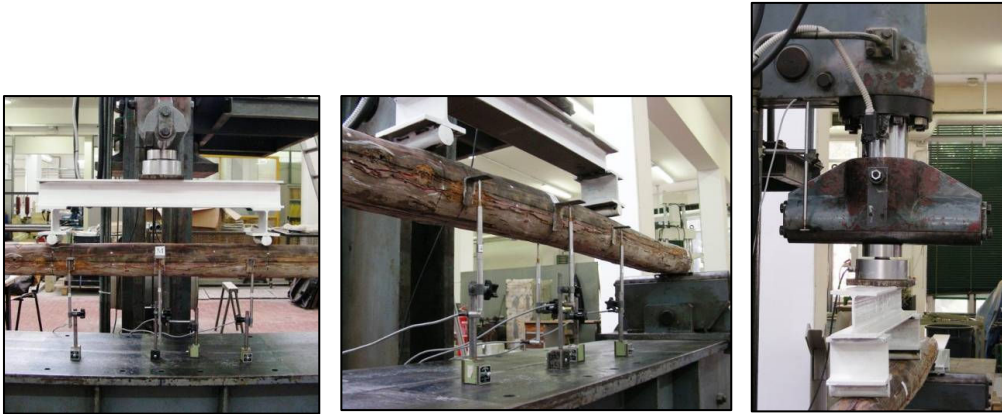
Figure 7.4. Bending tests on specimens type S_A-B – Testing equipment and set-up: displacement transducers (LVDTs) positioning.
