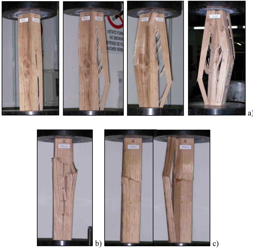
Figure 6.21. Compression tests parallel to grain on specimens type S_S\text{-C} – Typical collapse mechanisms: a) Propagation of longitudinal splitting; b) Wedge split; c) Shearing and splitting.
