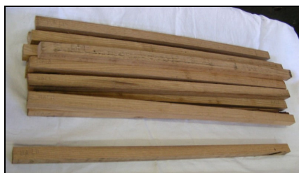
Figure 4.6. Tested specimens features – Defect-free specimens (DF): a) Extracted boards; b) Geometric features; c) Annual growth rings orientation with respect to the load direction. (continues)
