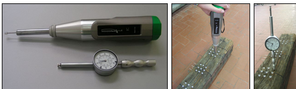
Figure 4.8. Non-destructive methods – Wood test hammer system: Wood Pecker device used in the experimental campaign.
