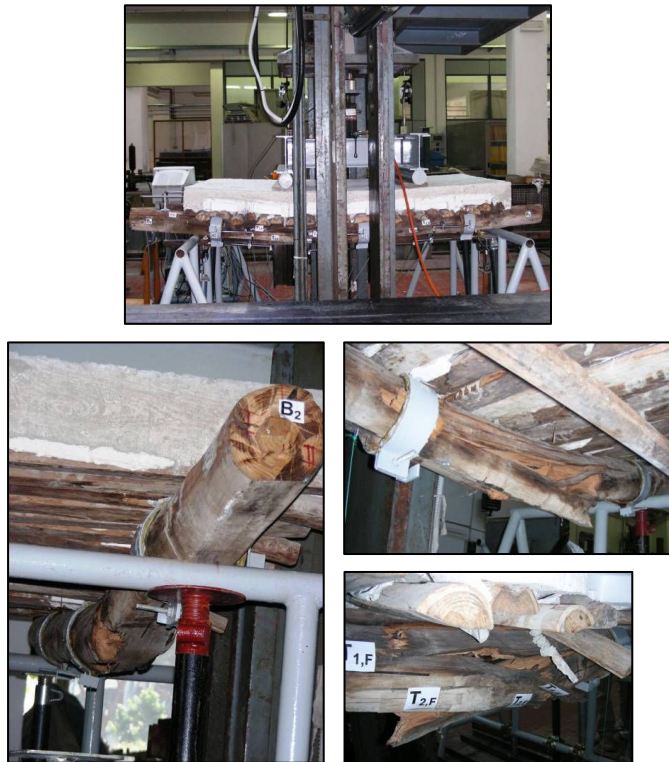
Figure 3.13. Bending test on composite floor: rupture mode.
