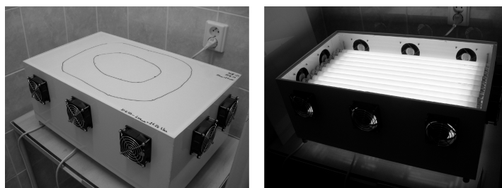
Figure 2. Irradiation device. Eleven L18W/30 lamps with maximum emission in the range of 530-620 nm are located under plastic diffuser sheet (Photo: L. Grada Kuliková).
