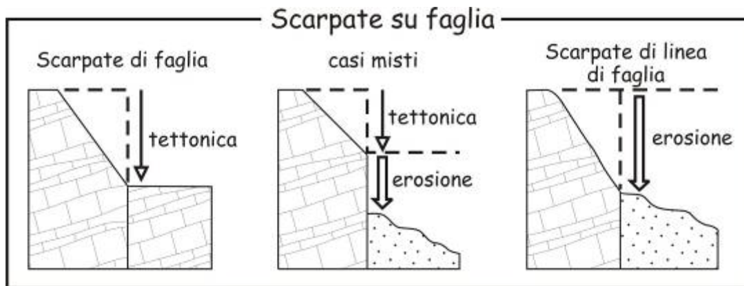
Fig. 2.2: scheme of the possible types of structural scarps (from Ascione and Cinque, 1997).
