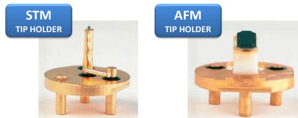
Figure 1.13: Omicron VT-AFM STM (left) and AFM(right)tip holder
