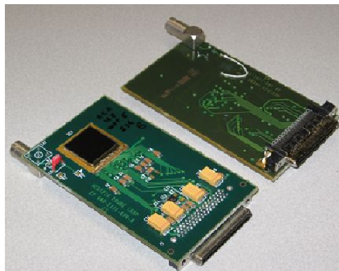
Fig. 2-2 Front and back of the Medipix2 hybrid detector.
