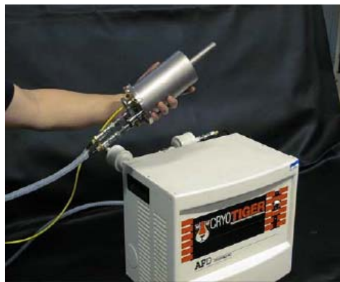
Figure 18: Example of cryocooler applied in aircraft wheels inspection.
