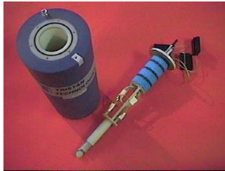
Figure 22: (left) cryogenic dewar, (right) cryogenic insert with the SQUID magnetometer at the bottom.
