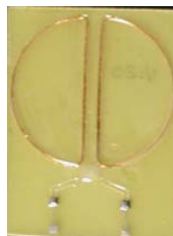
Figure 29: picture of a 2-D coil, made of copper wire.
