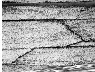
Figure 21: Schematization of the impacted cross-ply CFRP at energy less than 1J (up). the delamination arises inside the sample and is confirmed by a microscopic inspection (down) [15].
