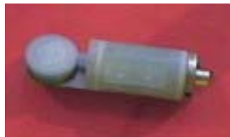
Figure 23: picture of the HTS dc- SQUID magnetometer used in this work.
