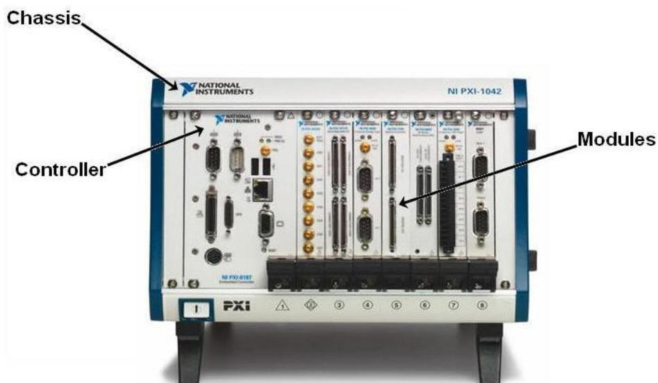
**Figure A-1: A standard 8-Slot PXI chassis with an embedded system controller and seven peripheral modules**
