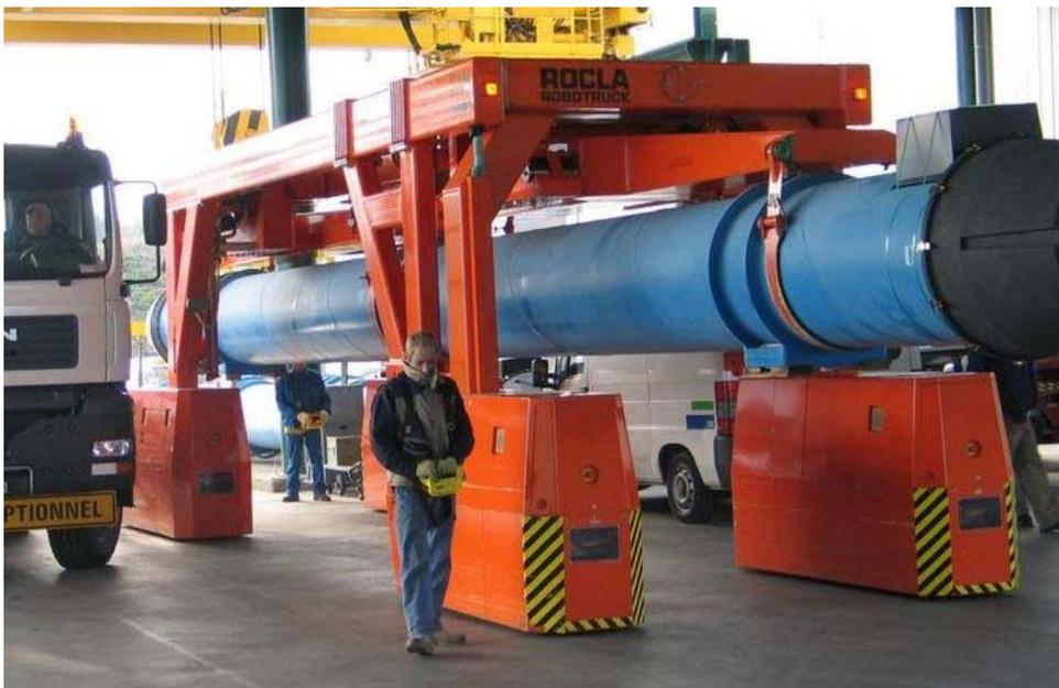
**Figure I-3** A LHC dipole magnet being transported to the test benches.
