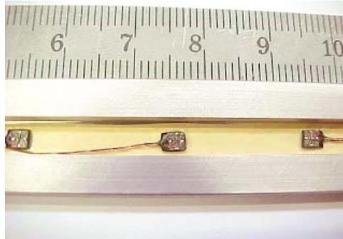
**Figure II-12 Axial unpackaged Hall Plates from AREPOC, type HHP-NU used in the existing Hall detector.**
