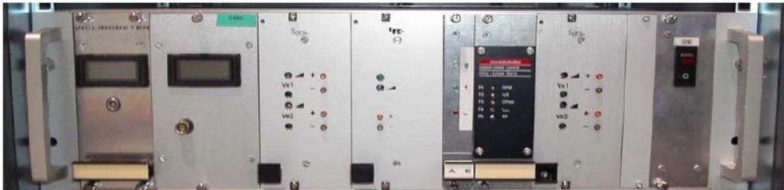
Figure VI-6: The front panel of the polarimeter electronic rack. (from left to right: the voltmeter for the tilt sensor, 50 mA hall plate supply, and, finally the power supplies for rack, DC motor, tilt sensor, stepping motor).
