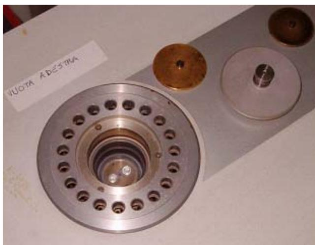
Figure 49. Sample and reference crucibles inside the measuring cell of the NETZSCH DSC 200 instrument.
