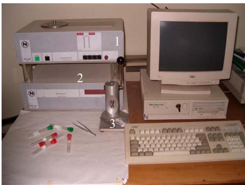
Figure 47. Computer assisted NETZSCH DSC 200 instrument 1: measuring part (with heating system and measuring cell), 2: controller, 3: sealing press.
