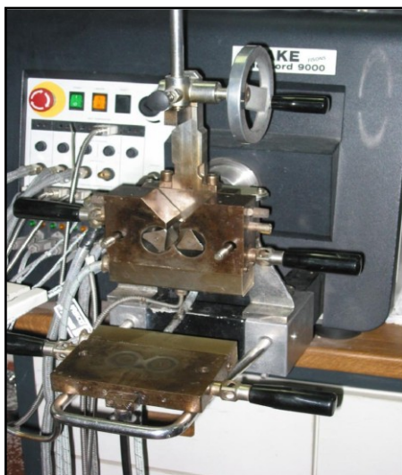
Figura 3.9 - Miscelatore HAAKE RHEOCORD RHEOMIX 600.
