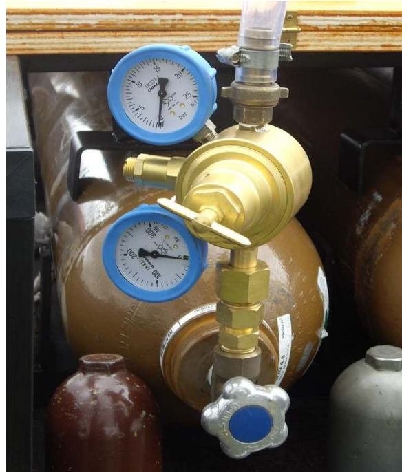
Figure IV-42 Pressure regulator mounted on the cylinder valve during inflation.
