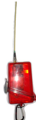
Figure IV-13 Altitude monitoring system: land receiver (left) and APRS transmitter (right).
