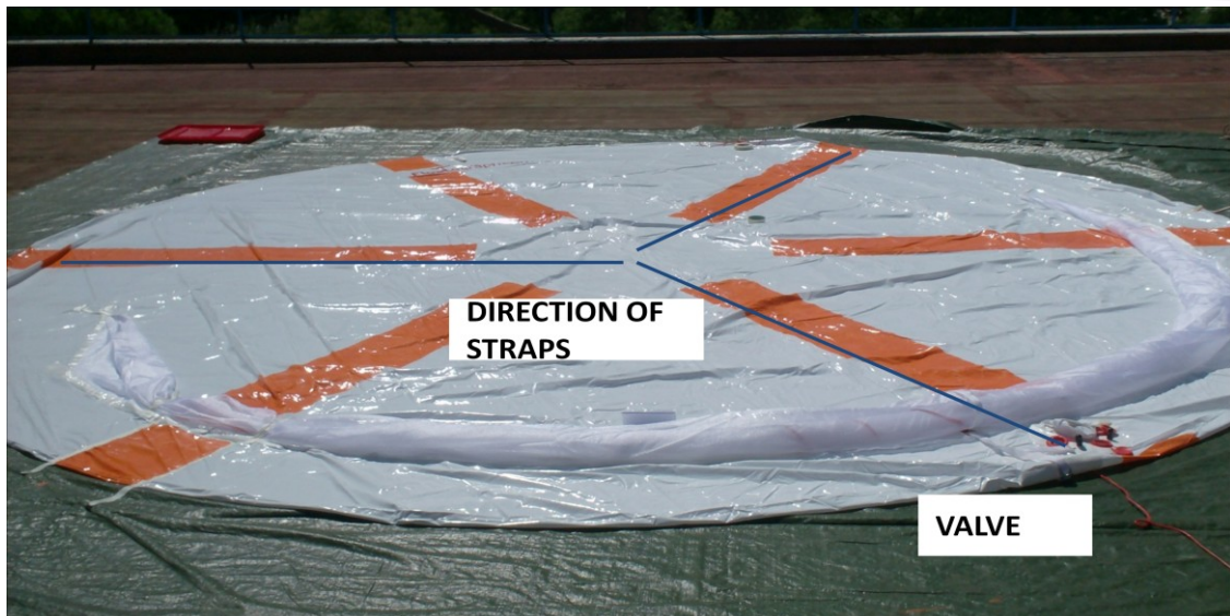
Figure IV-16 Front view of the upper surface of the kytoon. The direction of harness straps are put in evidence. The helium valves can be seen.
