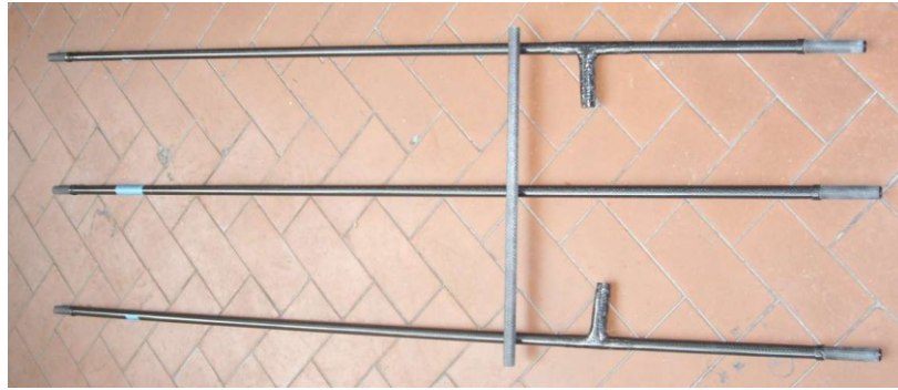
Figure IV-25 From the top: left front tube, back tube, front tube. The nacelle support tube spans between the others.
