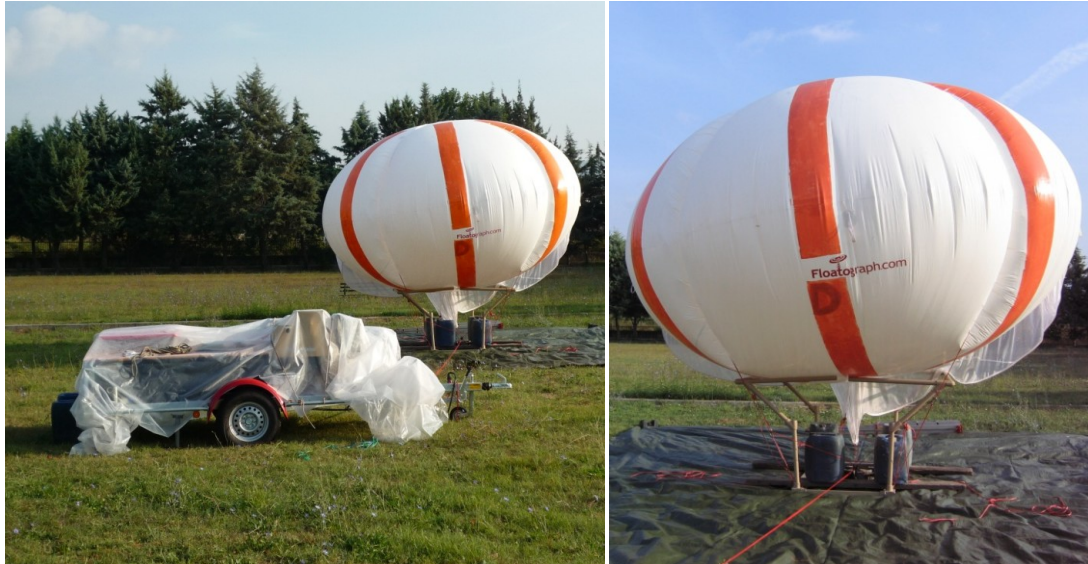
Figure IV-49 Garaging of the balloon (left) on the collapsible cradle (Right).
