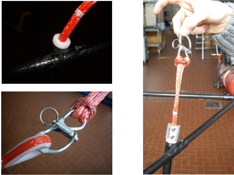
Figure IV-28 (Right) Holding bridle in position: the stopper blocks the bridle, while the snap hook links the bridle to the control lines (bottom left); circular plastic sleeves (top left).
