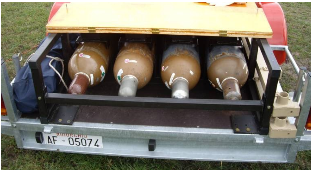
Figure IV-41 Open back end of the gas cylinder cage. The stopper bar is visible and the cylinder caps are pushing against it. The swiveling back end of the planking is open to permit access to the cylinders.
