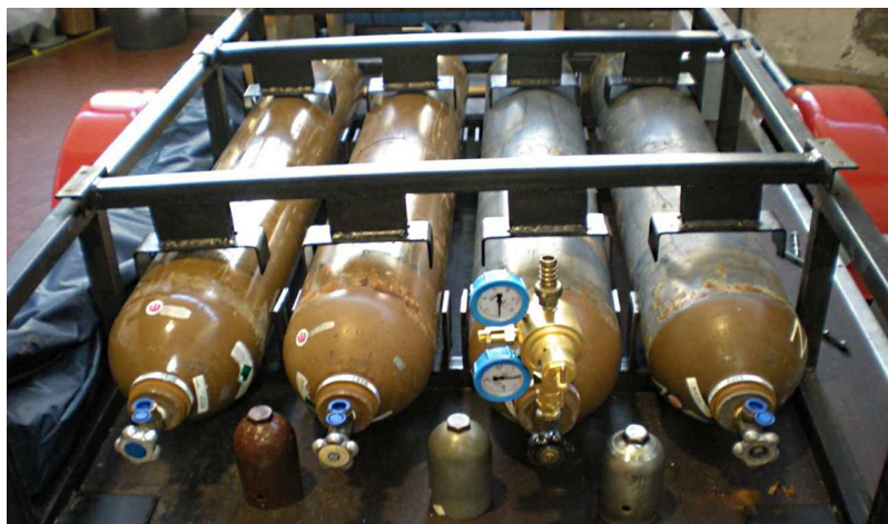
Figure IV-39 Loaded gas cylinder cage. The upper blocking bars are visible.
