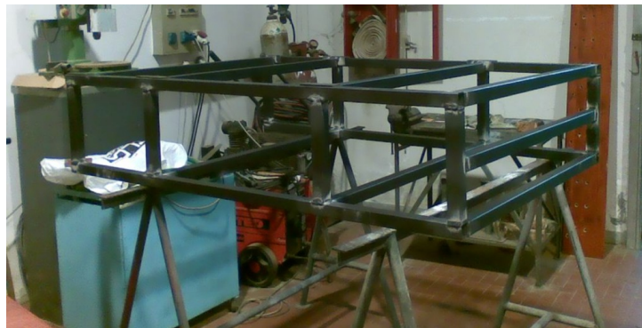
Figure IV-38 Gas cylinder cage after welding of the bars. The support platforms and the gas cylinders supports are still missing at this stage of setup.
