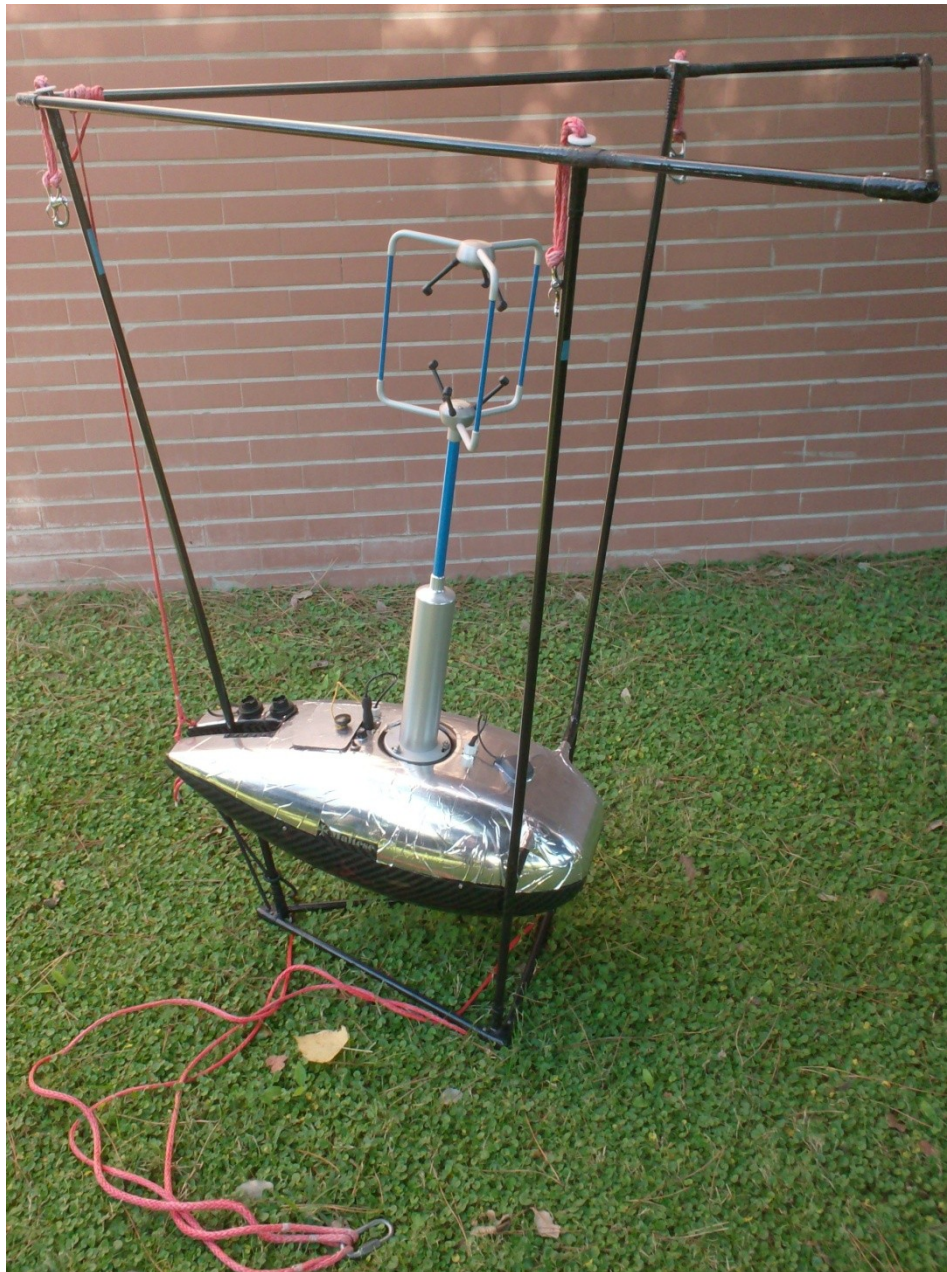
Figure IV-24 CATFISH gondola: they are visible the Gill Windmaster anemometer and the GPS's antenna (black rhomboid object); silver tape cover the CATFISH's body to surely avoid over heating due to the sun light. It can be seen the cable to regulate AoA of the nacelle.
