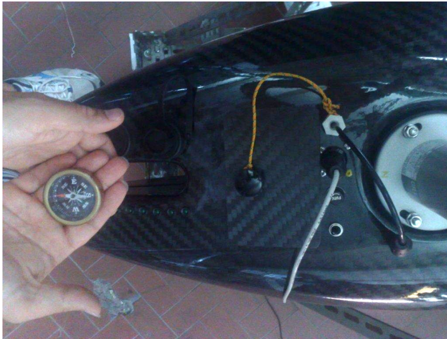
Figure VI-6 Magnetometer Calibration: x-axis of DEV coordinate system (line between the Nord spar on anemometer's mounting flange and the yellow screw's head) is aligned with magnetic Nord fixed by compass; IG 500N device connected to external PC via USB connection cable (white).
