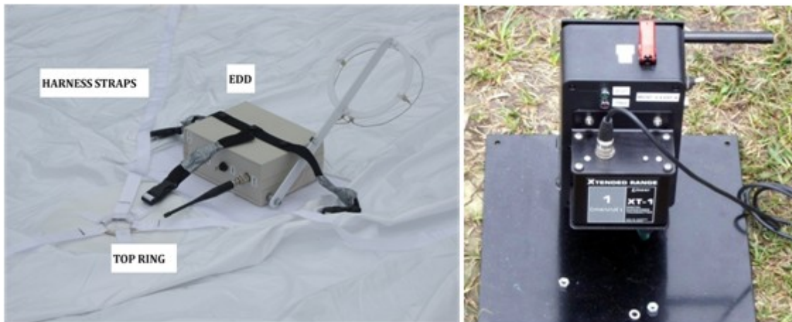
Figure IV-18 (Left) EDD kytoon unit. The actuated arm with the circular electrical resistance is shown on the left. EDD land unit (Right).
