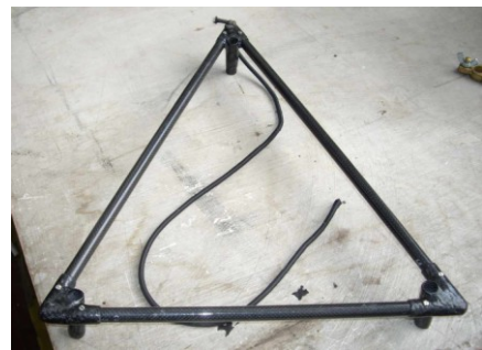
Figure IV-26 Lower triangular chassis. The elastic cable which is normally linked to the nacelle's back, can be seen.
