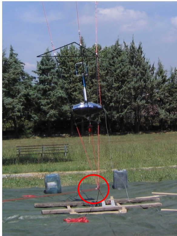
Figure V-13 Kytoon bounded trough the pulley (Red circle).
