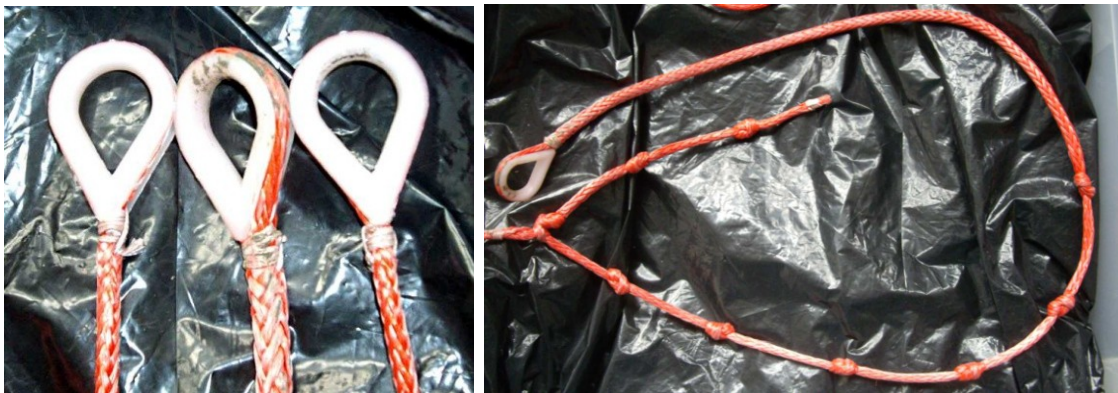
Figure IV-17 Loops at the ends of the control line, which are connected to the payload (left). Detail of the keel line and its knots. Notice that the line is set on the 3rd knot, which gives an AoA of 0^\circ (right).
