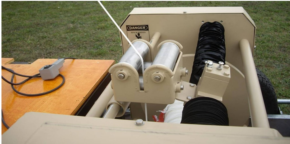
Figure IV-46 Winch in operation during a test flight. The roller fairlead is in the center.
