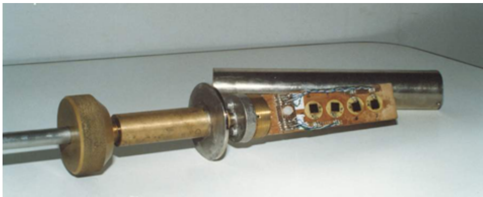
Fig.4.1 Picture shows end of special insert where SQUID containing chip mounted. The strip has 4 SQUID positions at both sides.
