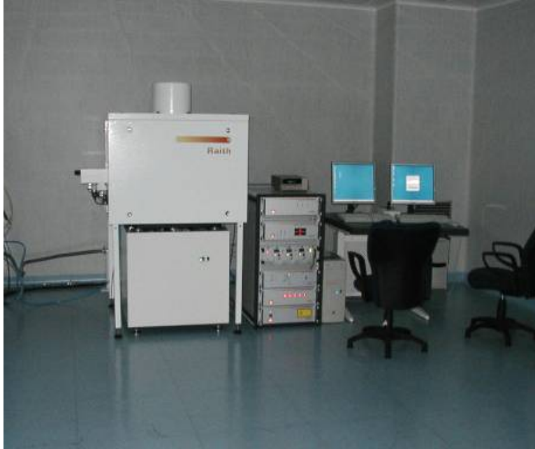
Fig.3.4 Picture of Raith E-beam system available in (CNR-ICIB) Institute of Cybernetics, CNR, NA, Italy
