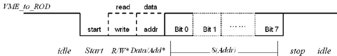
**Figure 41** – Addressing the destination register on the ROD FPGA.
