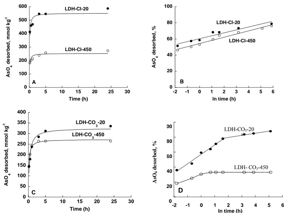
**Fig.25.** Kinetics of desorption of arsenate ( $\text{AsO}_4$ ) by phosphate ( $\text{PO}_4$ ) on LDH-CI-20 and LDH-CI-450 (A and C) and on LDH-CO<sub>3</sub>-20 and LDH-CO<sub>3</sub>-450 (B and D). In (C) and (D) the kinetics of desorption are described according to Elovich model.
