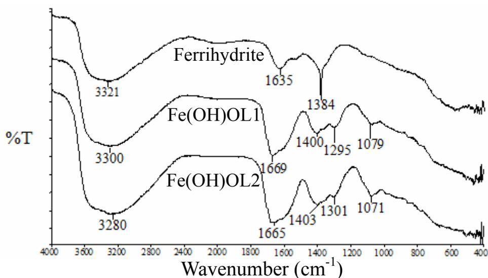
**Fig.4.** FTIR spectra of ferrihydrite and organomineral complexes
