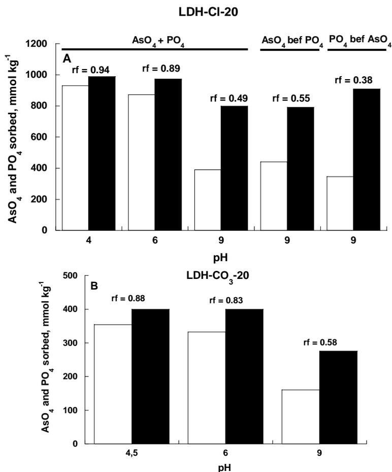
**Fig.24.** Amounts of arsenate (AsO<sub>4</sub>) and phosphate (PO<sub>4</sub>) sorbed on LDH-CI-20 (A) and LDH-CO<sub>3</sub>-20 (B) at pH 4.5, 6.0 and 9.0 when the two oxyanions were added as a mixture (AsO<sub>4</sub> + PO<sub>4</sub>) or by adding AsO<sub>4</sub> 3 h before PO<sub>4</sub> (AsO<sub>4</sub> bef PO<sub>4</sub>) or vice versa (PO<sub>4</sub> bef AsO<sub>4</sub>). rf stands for AsO<sub>4</sub> sorbed/PO<sub>4</sub> sorbed molar ratio
