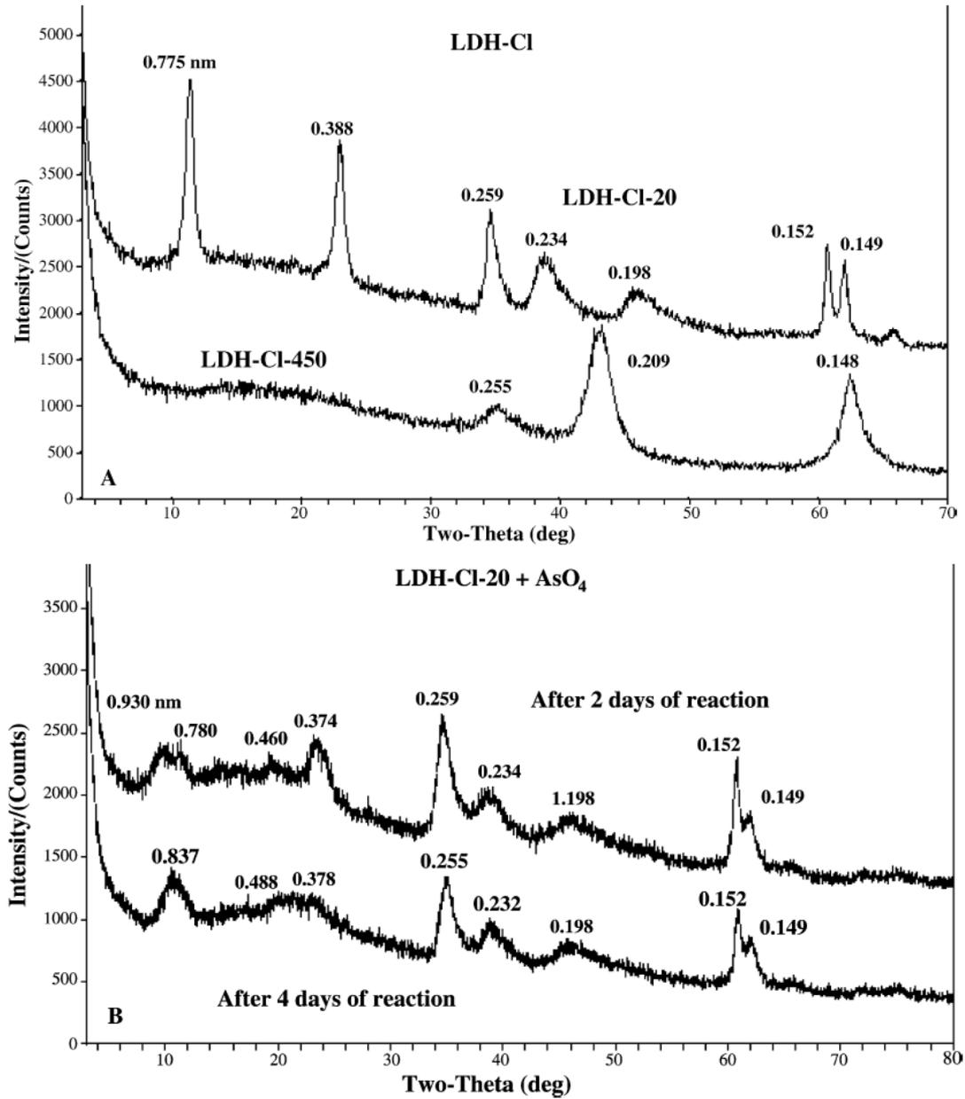
**Fig.20.** Powder X-ray diffraction patterns of LDH-CI (A) and LDH-CI after addition of arsenate at pH 6.0 ( $1400 \text{ mmol kg}^{-1}$ ) after 2 days or 4 days of reaction (B)
