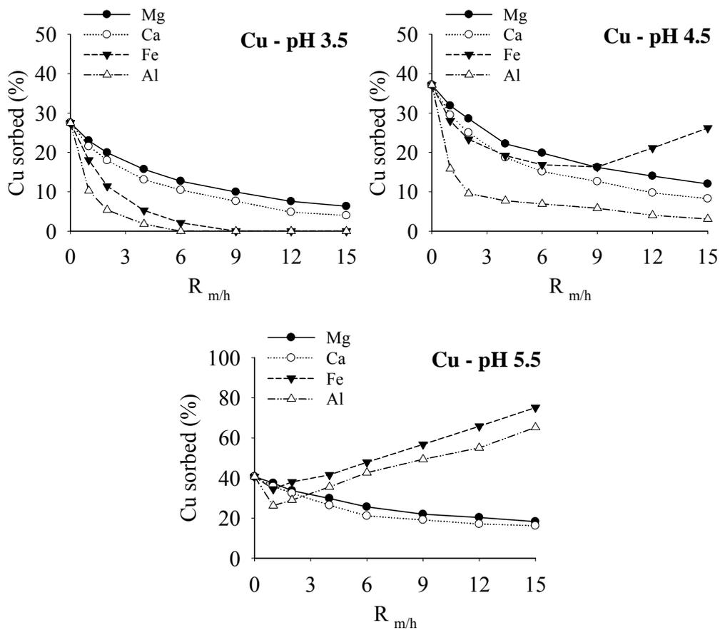
**Fig.17.** Effect of concentration of Al, Fe, Ca and Mg on the sorption of Cu by Na-montmorillonite at pH 3.5, 4.5 and 5.5
