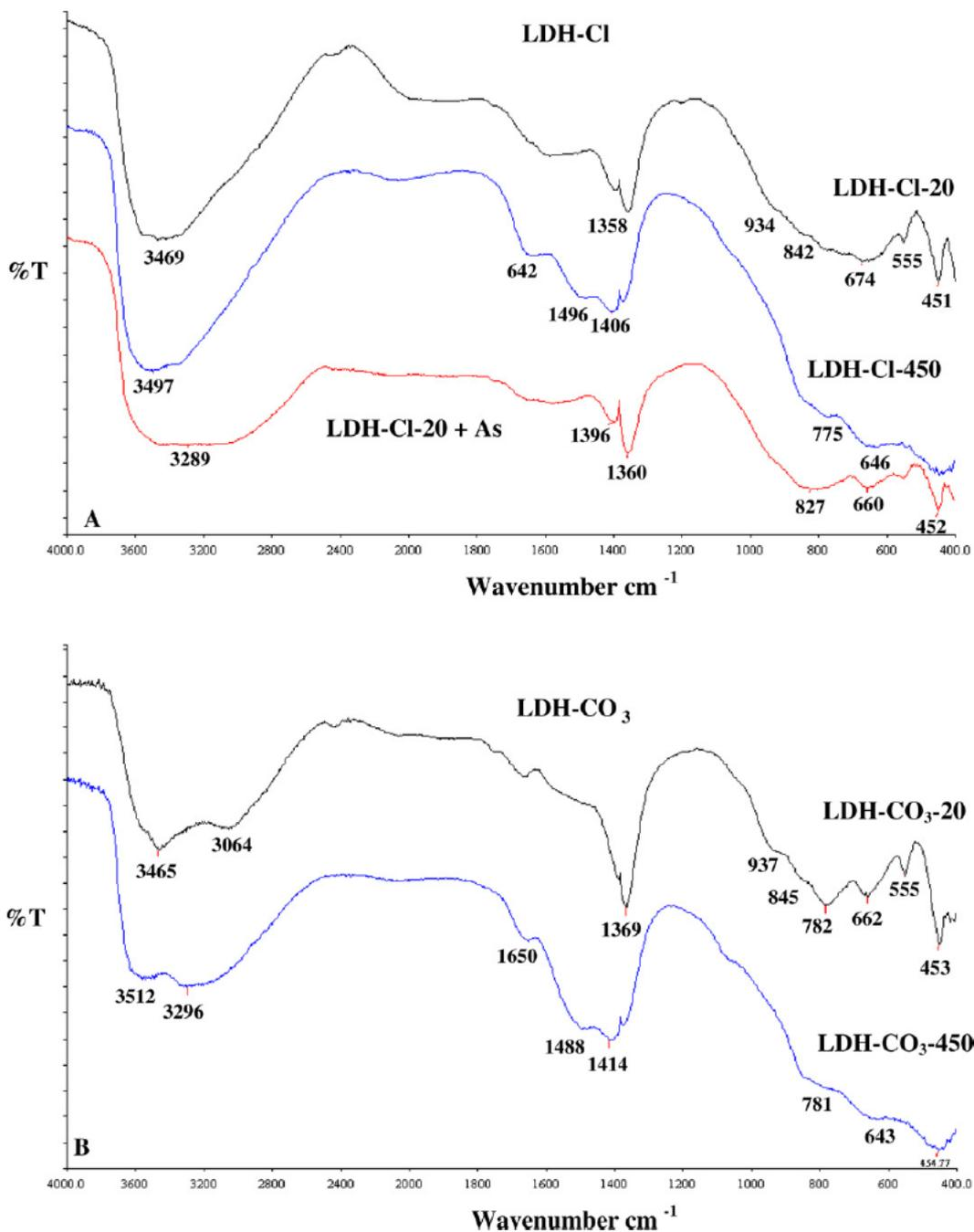
**Fig.21.** FTIR spectra of LDH-CI (A) and LDH-CO<sub>3</sub> (B) minerals
