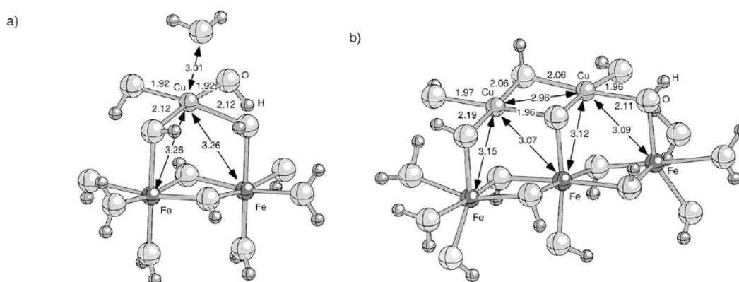
**Fig.2.** Bidentate corner-sharing mononuclear surface complex (a) and tridentate corner-sharing binuclear surface complex of Cu formed on goethite, hematite and lepidocrocite (Peacock and Sherman, 2004)
