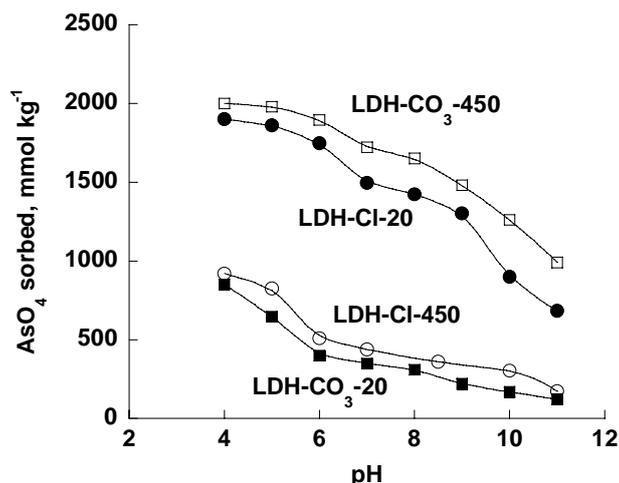
**Fig.23.** Effect of pH on the sorption of arsenate ( $AsO_4$ ) on uncalcined (LDH-CI-20 and LDH-CO<sub>3</sub>-20) and calcined (LDH-CI-450 and LDH-CO<sub>3</sub>-450) minerals
