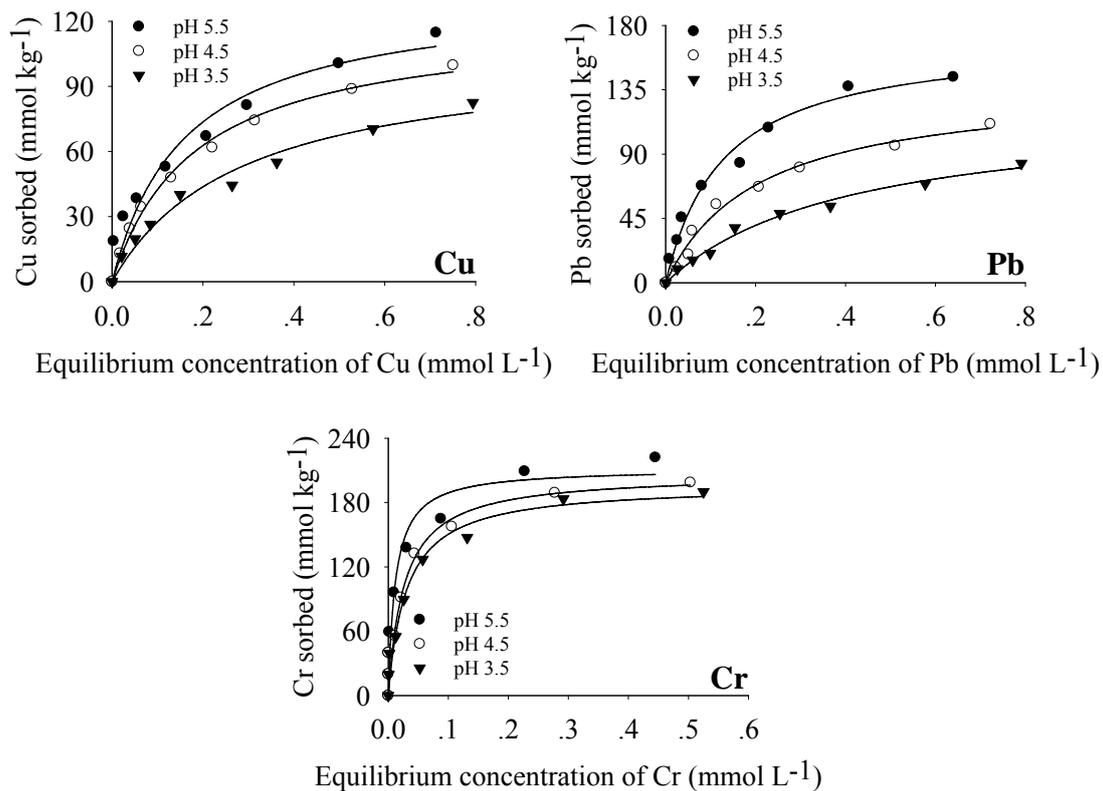
**Fig.15.** Langmuir sorption isotherms of Cu, Pb and Cr on Na-montmorillonite at pH 3.5, 4.5 and 5.5
