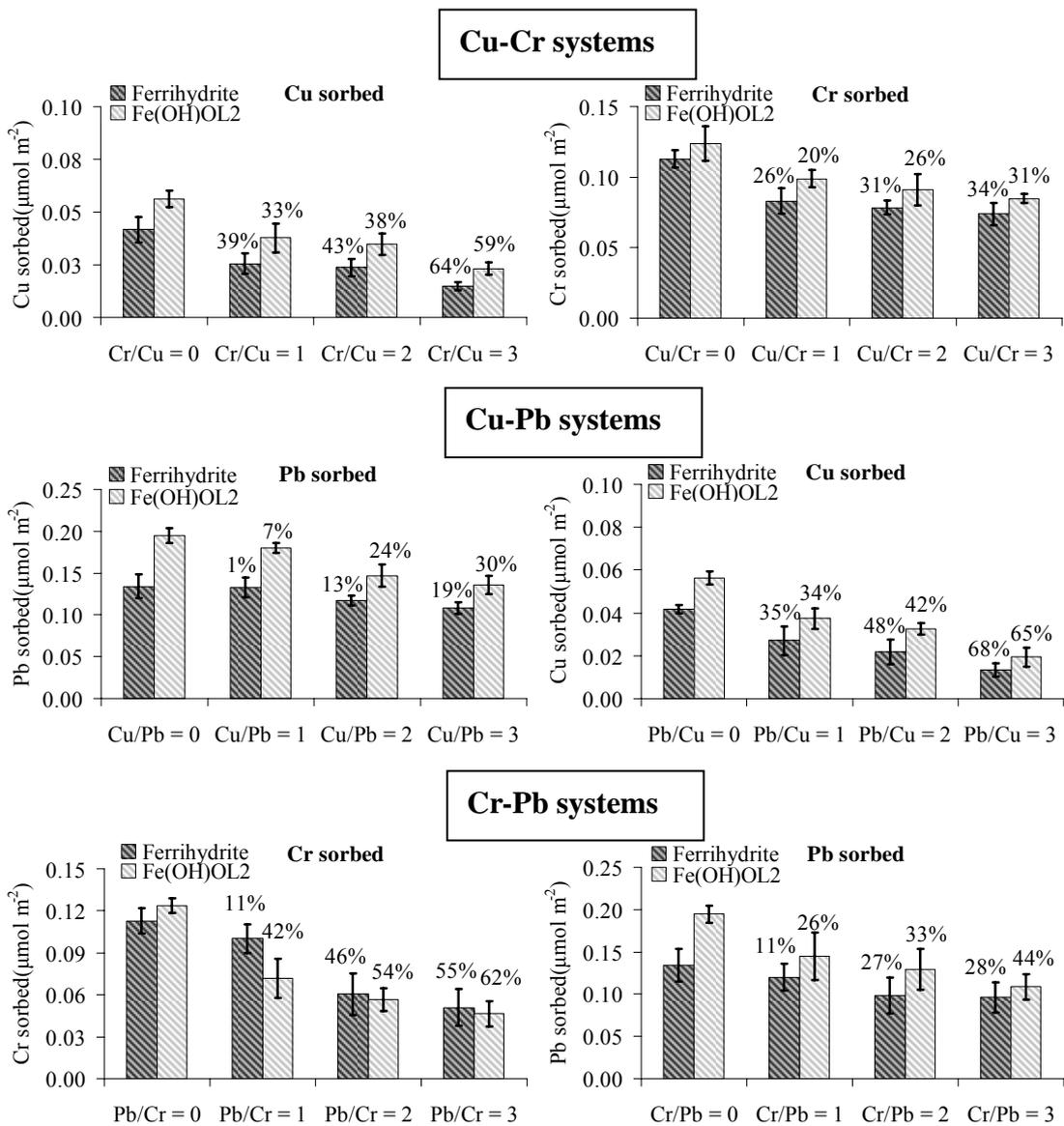
**Fig.8.** Amounts of Cu, Cr and Pb (M1) sorbed on ferrihydrite and Fe(OH)OL2 at pH 4.5 in the absence or presence of increasing concentration of a competing metal (M2) in binary systems (Cu-Cr, Cu-Pb or Cr-Pb) at initial M2/M1 concentration ratio of 0, 1, 2, and 3. The percentage values on the columns indicate the inhibitive efficiency of M2 in preventing M1 sorption.
