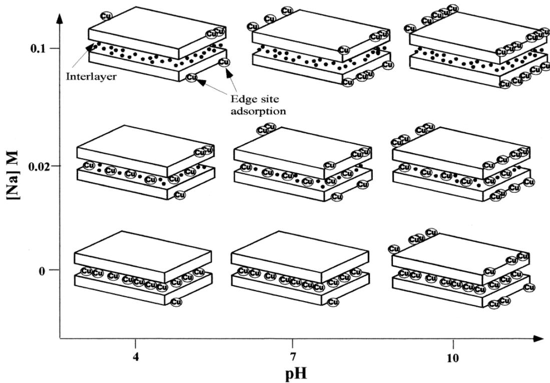
**Fig.1.** Schematic illustration of the effect of pH and Na concentration on the distribution of adsorbed copper on the permanent charge interlayer and edge sites of montmorillonite (Morton et al., 2001)
