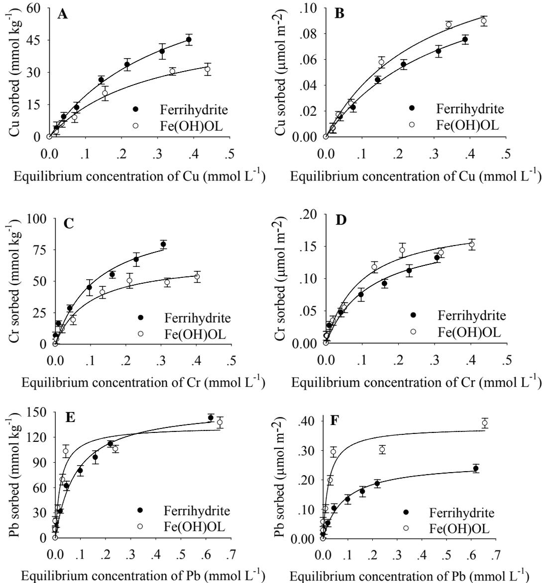
**Fig.6.** Sorption isotherms of Cu, Cr and Pb on ferrihydrite and Fe(OH)OL2 at pH 4.5.
