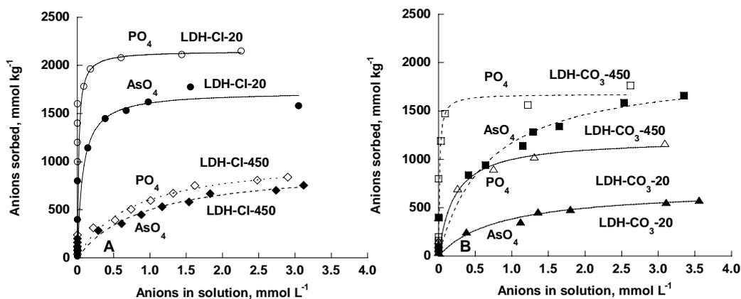
**Fig.22.** Sorption isotherms at pH 6.0 and 20 °C of arsenate ( $\text{AsO}_4$ ) and phosphate ( $\text{PO}_4$ ) onto uncalcined (LDH-Cl-20 (A) and LDH- $\text{CO}_3$ -20 (B)) and calcined (LDH-Cl-450 (A) and LDH- $\text{CO}_3$ -450 (B)) minerals
