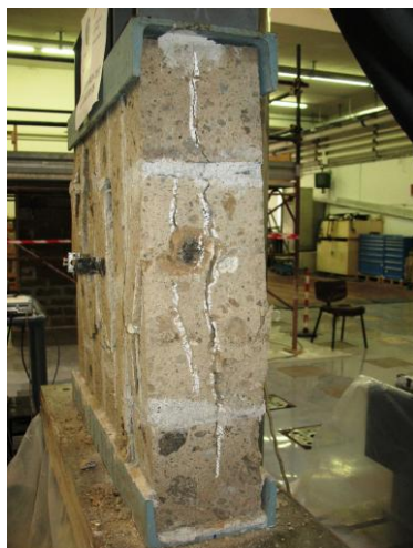
Figure A.5 Transverse splitting of a specimen
