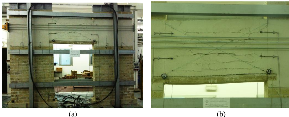
Figure C.10 (a) Near-collapse state of the repaired wall; (b) damage to the spandrel panel
