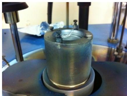
**Fig. 3.14 Ion Gun source - University of Naples "Federico II".**
