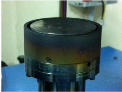
Fig. 3.2 Magnetron sputtering (Py target) - University of Naples "Federico II".
