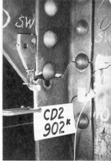
Figure 3.26 Angle failure in built-up section (Kulak et al., 1987).
