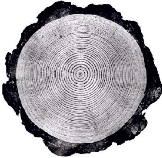
Figure 2. Cross section showing growth rings
