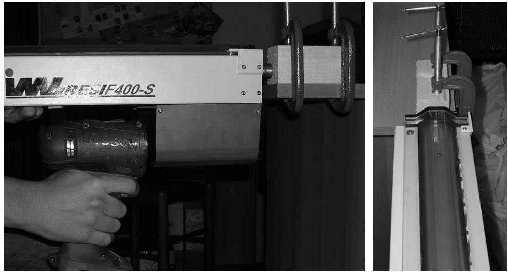
Figure 1. Spruce samples subjected to Resistographic analysis in longitudinal direction.
