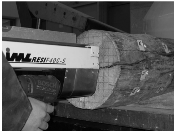
Figure 2. A Resistographic analysis in longitudinal direction.
