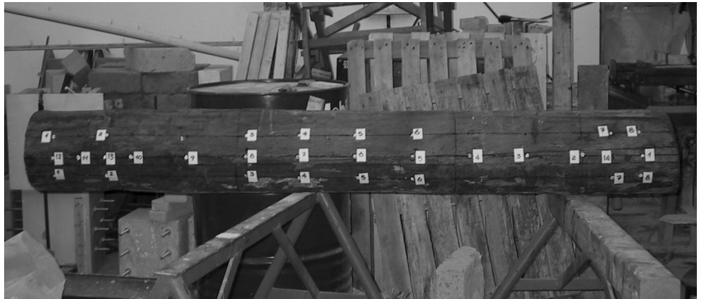
Figure 3. The transversal Resistographic analyses carried out on the whole beam.
