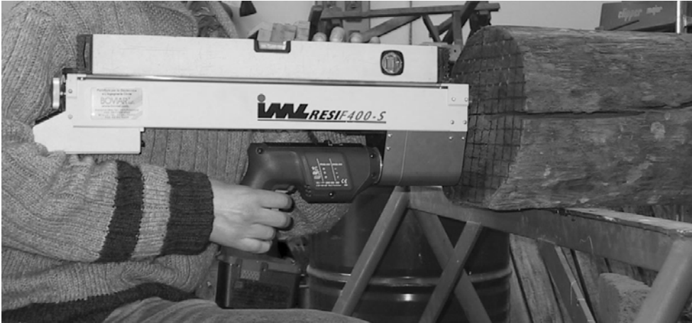
Figure 1. the Resistograph during the NDT campaign.
