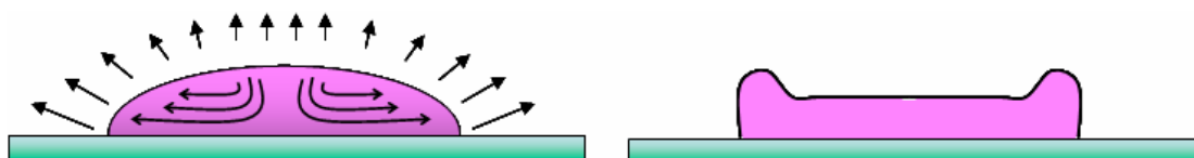
Figure 1.13 Illustration of “coffee-stain” effect. Evaporation rate (represented by upward arrows) is highest at the edges of a printed droplet resulting in an accumulation of the solute at the periphery at the end of the drying process.
