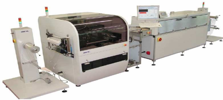
Figure 1.10 Image of the inkjet printing equipment at ENEA Portici.
