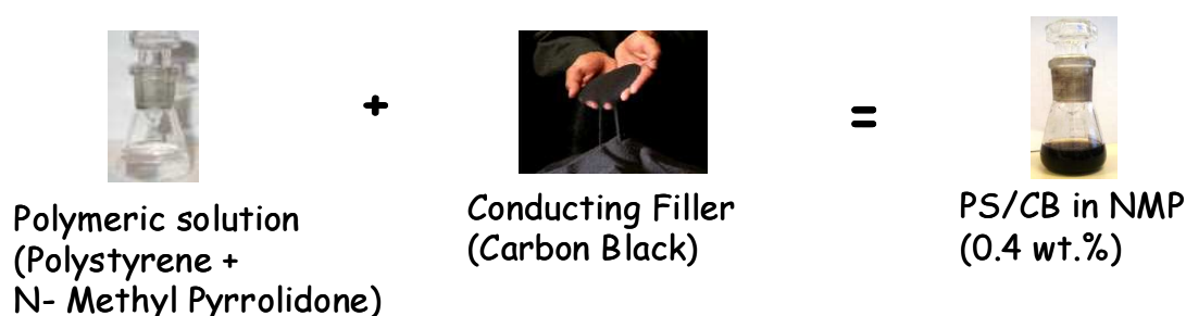
Figure 2.2 Ink preparation: the polystyrene was dissolved in NMP and the Carbon Black was dispersed in the polymeric solution.
