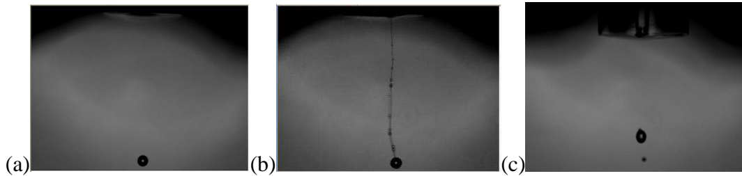
Figure 1.11 Drop images of a stable condition (a), formation of filament (b) and formation of satellite droplet (c).
