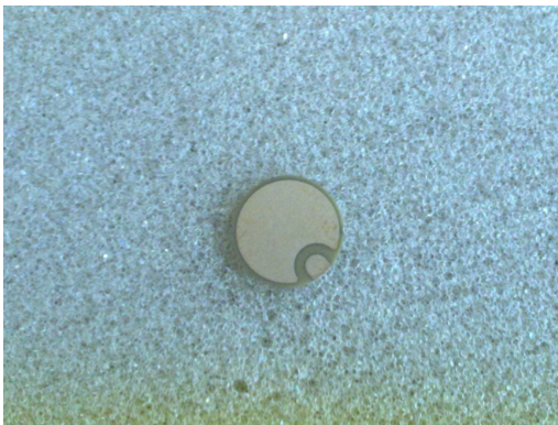
Fig. 1.3a - PWAS disk transducer.
