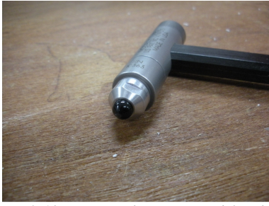
Fig 2.19 – Impact hammer used for the test: PCB Electronics mod. 086C03
