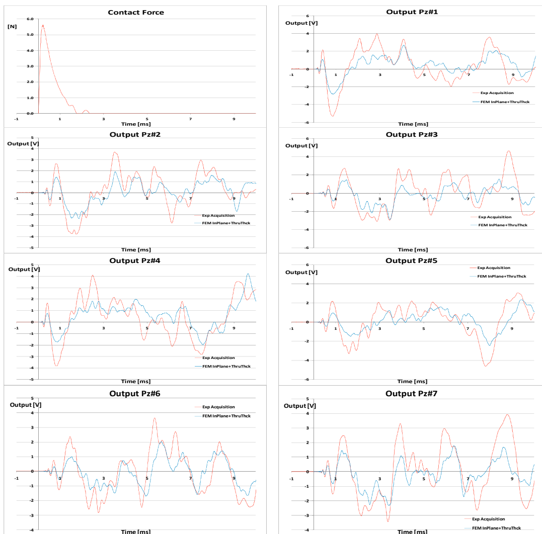
Fig 2.32 – Comparison between experimental data and FEM solution for the impact test on the NP130 plate
