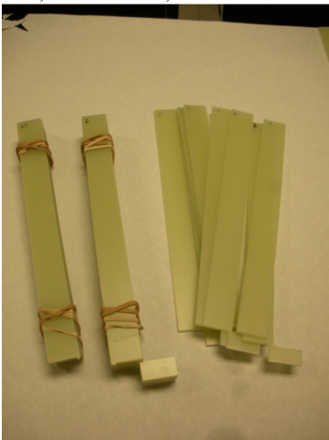
Fig. 1.22 – Specimens from NP130 according with Standard Tensile Test Method ASTM D-3039
