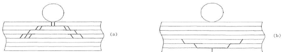
Fig 2.4 – Damage development in (a) rigid and (b) flexible targets
