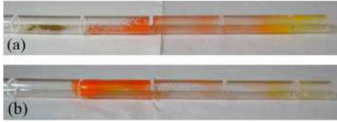
Figure 2-4: Comparison between the result of the growth of a) material as purchased, b) regrowth of the obtained crystals. Only in the first case impurities are present in correspondence of the section where the purchased powder was. This indicates that the growth procedure causes a purification of the crystals[95].
