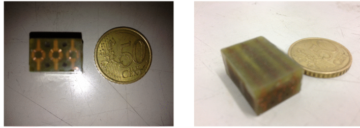
Figure IV.22: the modified \Omega -shape metamaterial structure used for LC tenability system.
