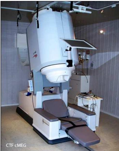
order synthetic gradiometers (29 references); the number of sensing channels is either 151 or 275. The Dewar orientation is adjustable between the vertical and horizontal positions.
