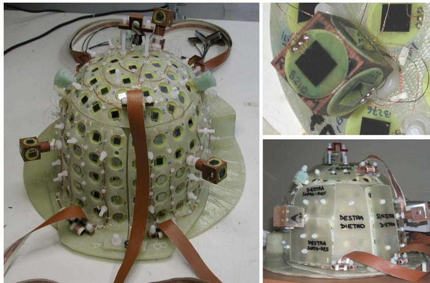
Figure 3.10 - The SQUID arrays in helmet shape containing 154 measurement channels and 9 reference sensors. On the right side: particular of a reference tower [top] and the helmet surrounded by the thin fiberglass shields [bottom]
