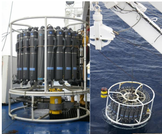
Figure 2.3 : Niskin bottles fitted on a rosette with CTD instrumentation.
