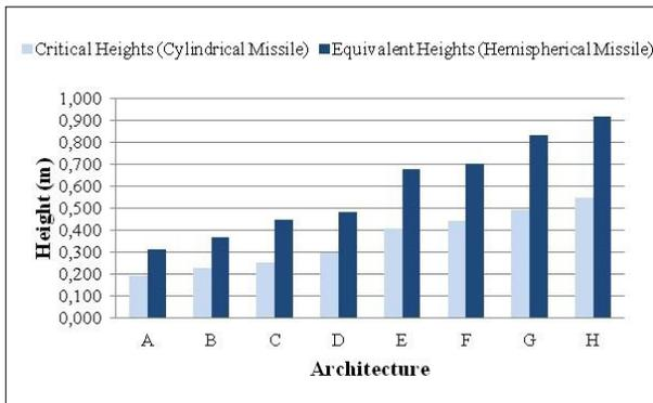
Fig. 3 Critical Heights (EN 913) compared to Equivalent Heights (EN 1177)
