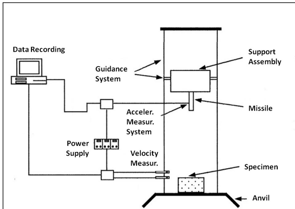
Fig. 2-12 Low-velocity Impact Testing Apparatus
