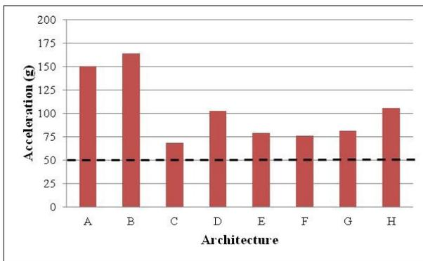
Fig. 4 Hemispherical Missile Accelerations measured from Equivalent Heights
