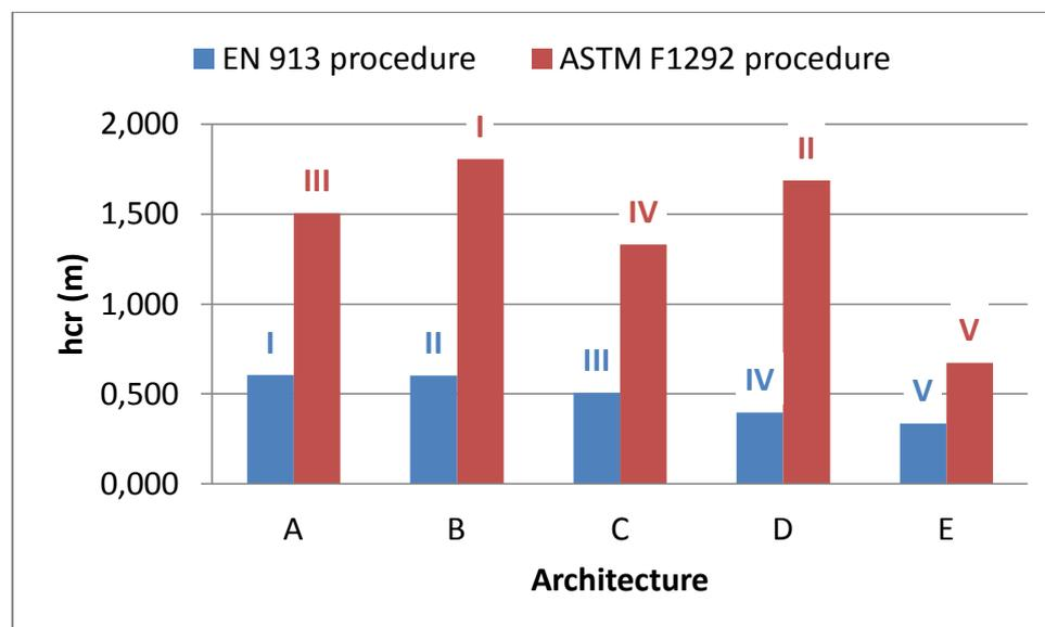
Fig. 3-2 Critical Fall height architectures performances according EN 913 and ASTM F1292 procedure
