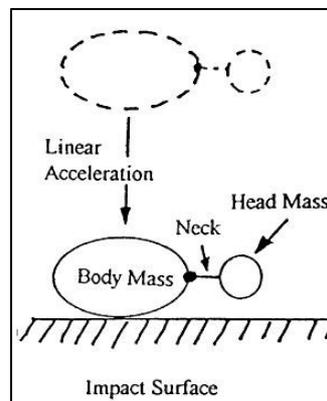
Fig. 2-5 Linear acceleration [10]
