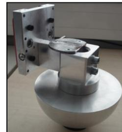
Fig. 4 Impact testing support assembly
