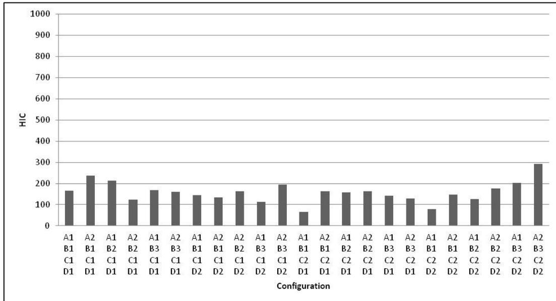
Fig. 3-5 HIC scores from equivalent drop heights
