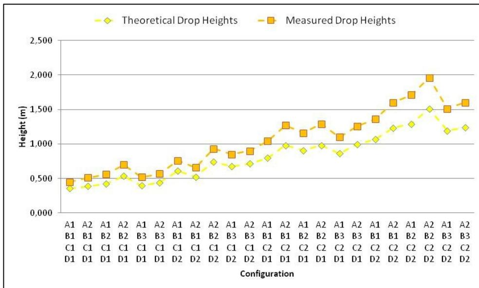
Fig. 3-7 Measured and Theoretical Drop Heights Comparison
