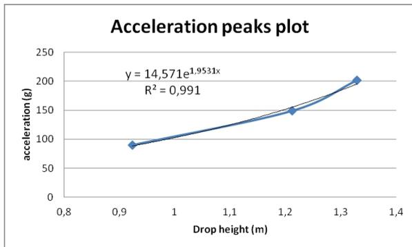
Fig. 8 Acceleration peaks vs drop height values plot
