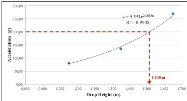
Fig. 7 Acceleration vs Drop height plot
