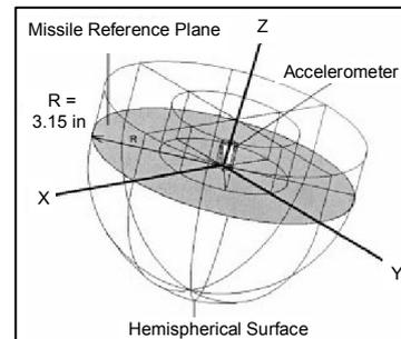
Fig. 4: ASTM Missile [6]
