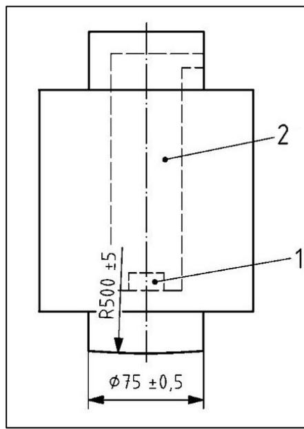
Fig. 2-16 Required Indenter: 1. Accelerometer; 2. Space for mounting the accelerometer
