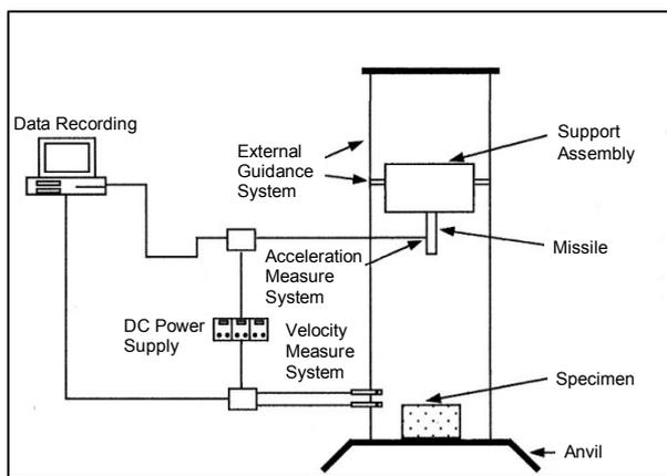
Fig. 1: General impact testing set-up
