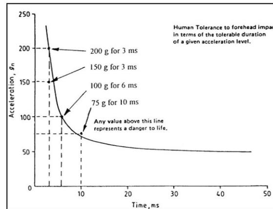
Fig. 2 Human tolerance to forehead impact in terms of the tolerable duration of a given acceleration level [7]
