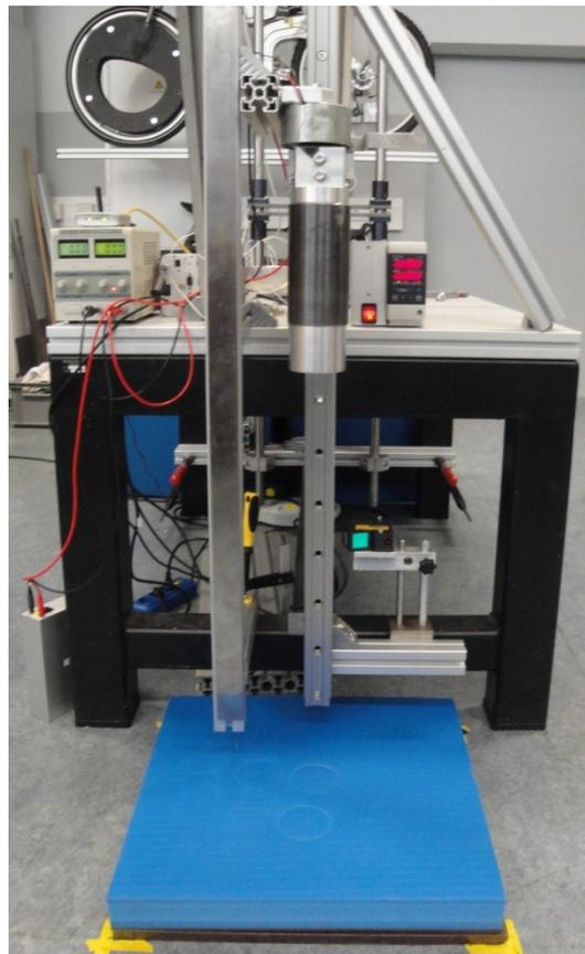
**Fig. 3-1 The working impact testing apparatus**
