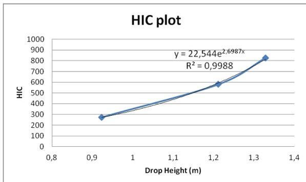
Fig. 9 HIC vs drop height values plot
