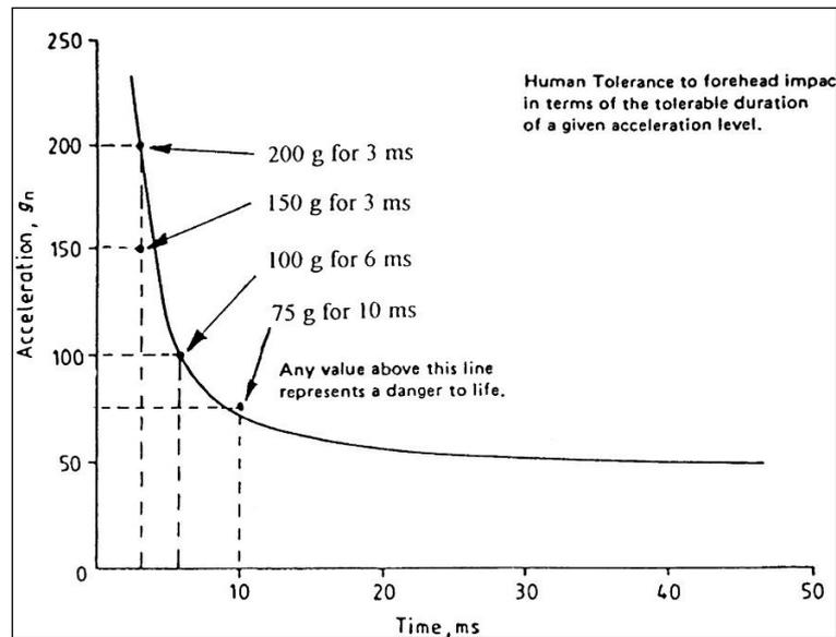
Fig. 2-9 Human tolerance to for head impact in terms of the tolerable duration of a given acceleration level
