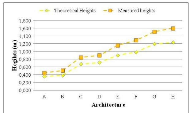
Fig. 6 Measured and Theoretical Drop Heights Comparison
