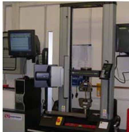
Figure 6.2 Experimental setup for tensile tests on rubber
