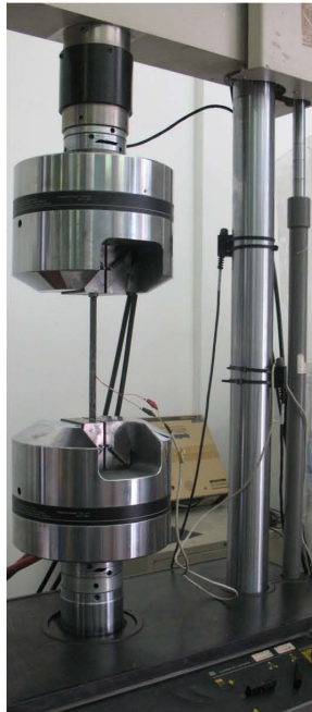
Figure 6.13 Universal testing machine used for tensile tests on FRP sheets.
