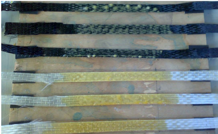
Figure 6.12 Production of FRP specimens for tensile tests.
