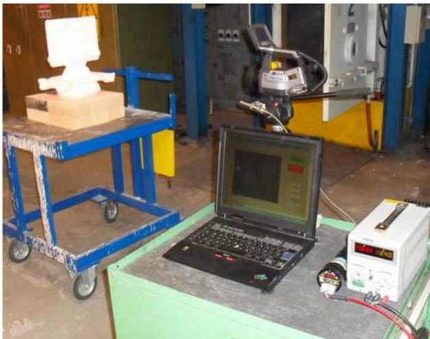
**Figure 4.3:** Experimental apparatus for EHT emissivity measurement.
