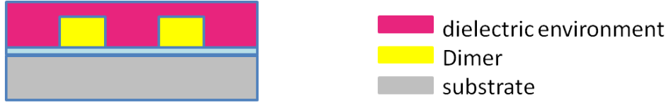
Figure 5.1: Cross section of the dimer in a dielectric environment(pink) of varying index.
