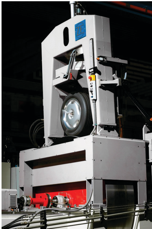
Figure VI.1 – The ZF machine to measure tire rolling resistance
