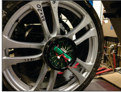
Figure III.15 - The I/O unit
