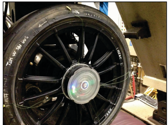
Figure III.17 - The thermo camera to acquire the surface temperature and the I/O unit fitted on the rim
