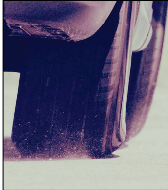
Figure II.12 – Tire deformation in corner
