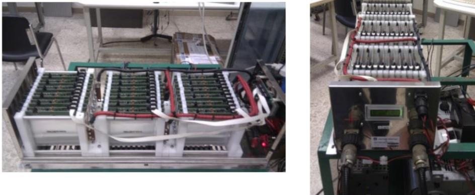
**Figure 3.27 – Prototype 30.5 F 136 V laminated LiC module of D.I.E.T.I.**
