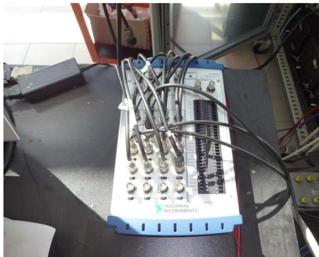
Figure 5.12 – Assembly view of the NI-DAQ 6229 usb DAQ
