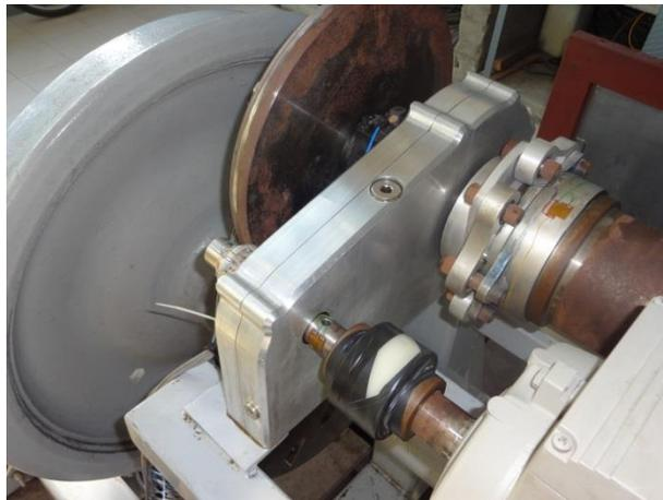
**Figure 5.4 – Particular of the dancing ring and the reduction unit**
