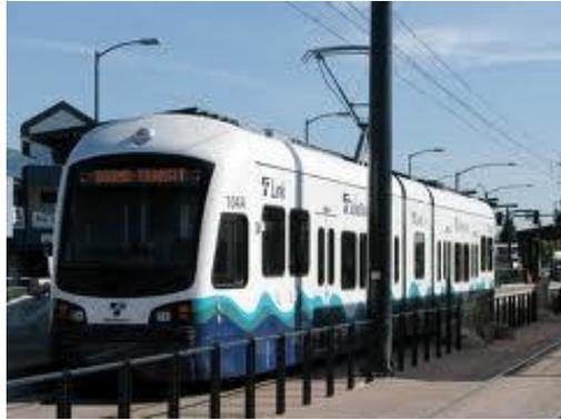
**Figure 1.5 - Overhead contact wires to power light rail system**
