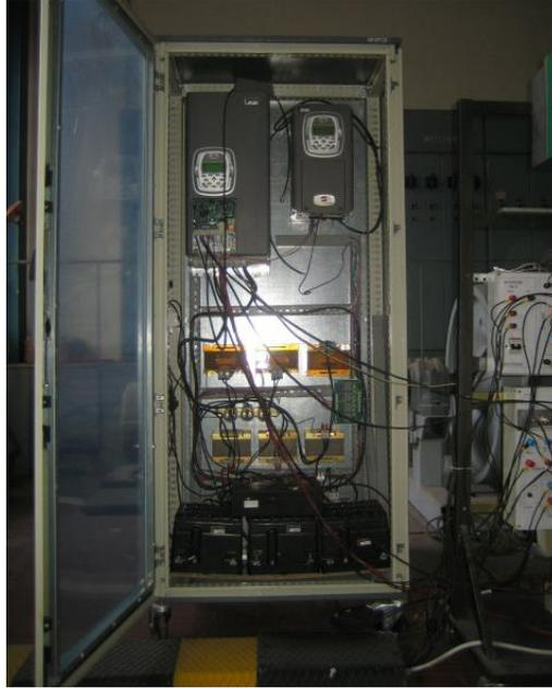
**Figure 5.11 – Frontal picture of the interleaved DCDC converter**
