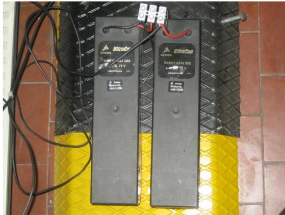
**Figure 3.42 - Picture of EPCOS 3.3 F 75 V SC modules of D.I.E.T.I.**
