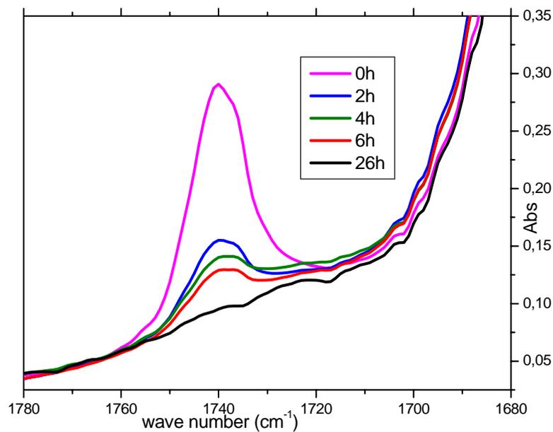
Figure(II)-21: Release of Jojoba Oil through polyamide matrix for polyamide 6/8.5 wt% nanjoj.
