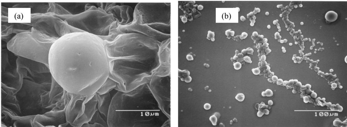
Figure (I)-10. SEM photomicrographs of microcapsules.
