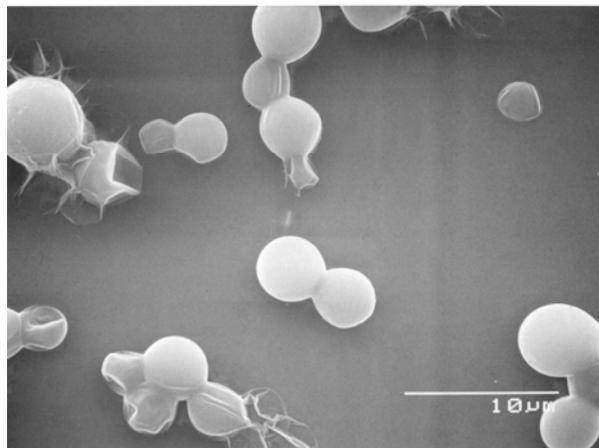
Figure (I)-20. SEM photomicrographs of microcapsules.
