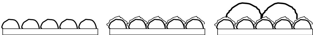
Fig.(I)-5: Nylon primary membrane formation and subsequent growth on the organic side
