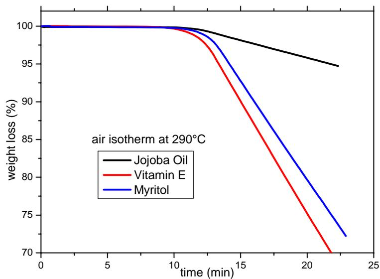
Fig.17: TGA isothermal in air
