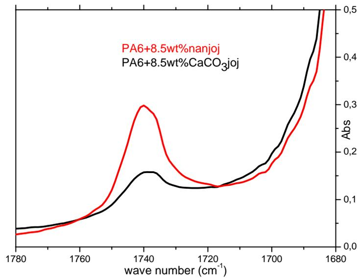
Figure(II)-24: Polyamide 6/organoclay-Jojoba and polyamide 6/ $\text{CaCO}_3$ -Jojoba sections at the same filler content
