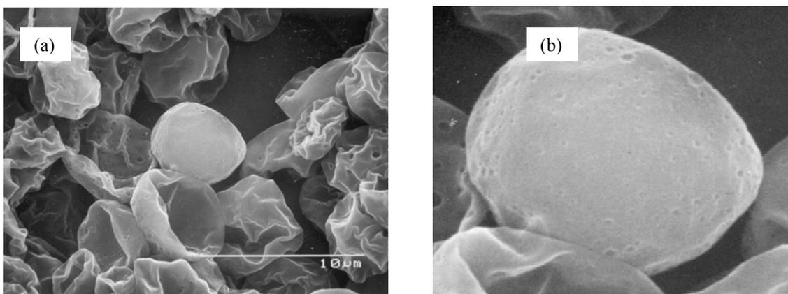
Figure (I)-12. SEM photomicrographs of microcapsules.
