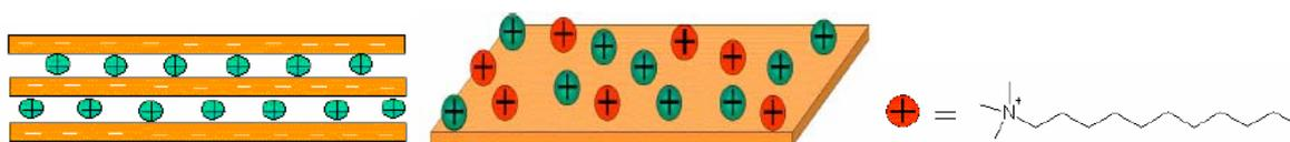
Figure (II)-2: Ion exchange with alkyl ammonium
