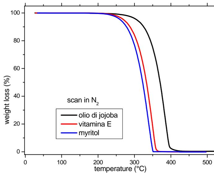
Fig.14: TGA scan in N<sub>2</sub>
