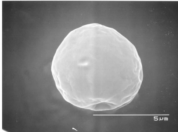
Figure (I)-15. SEM photomicrographs of microcapsules.
