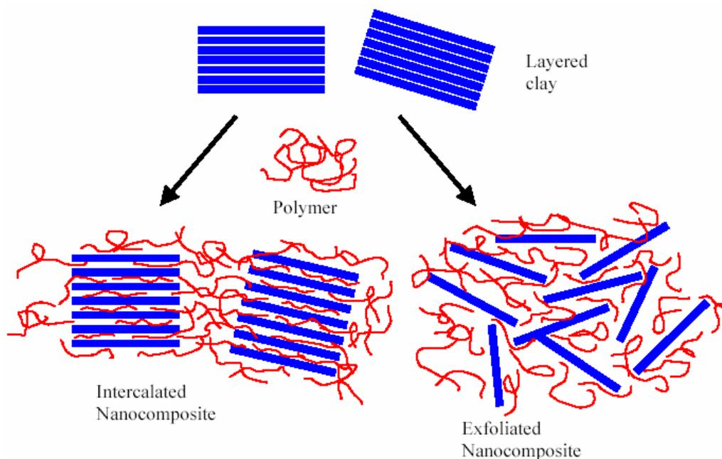
Figure(II)-3: Formation of intercalated and exfoliated nanocomposites from layered silicate and polymer
