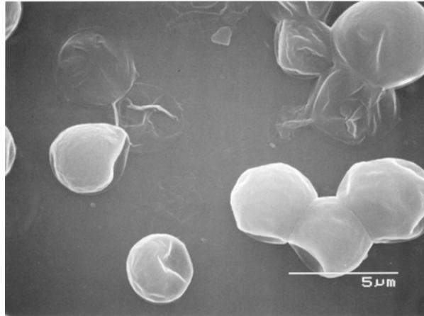
Figure (I)-17. SEM photomicrographs of microcapsules.
