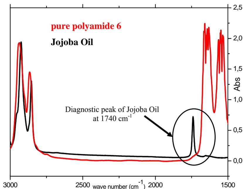
Figure(II)-6: Spectra overlap of pure polyamide 6 and Jojoba Oil
