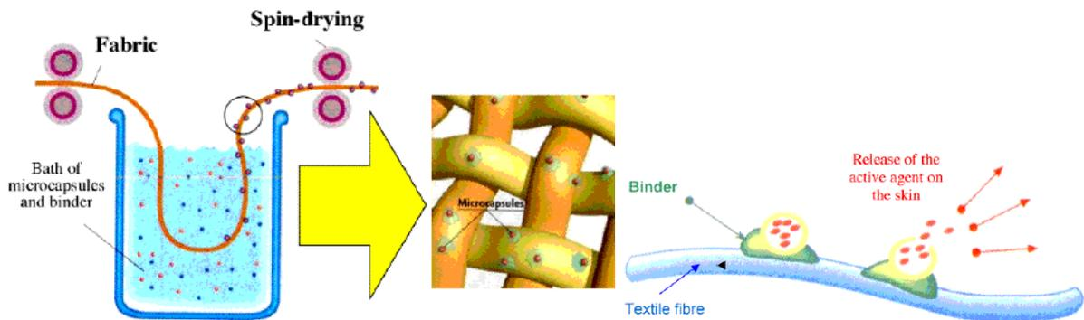
Fig.(I)-2 : example of microcapsules application on fabrics
