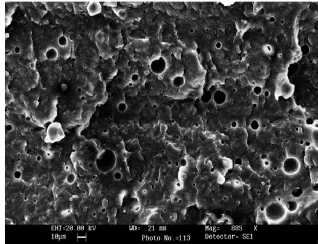
Figure (I)-25. SEM photomicrograph of PA6 matrix containing 5wt% microcapsules
