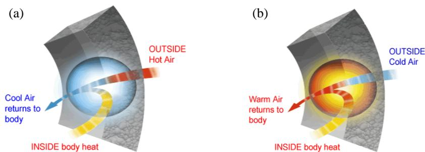
Fig.3: Heat exchange through fibers containing encapsulated PCM.
