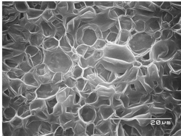
Figure (I)-18. SEM photomicrographs of microcapsules.
