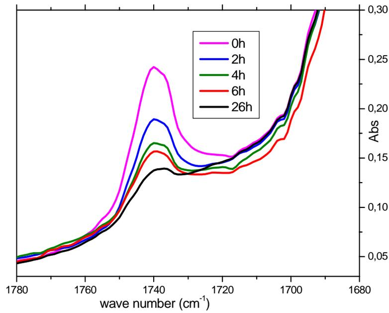
Figure(II)-20: Release of Jojoba Oil through polyamide matrix for polyamide 6/7 wt% nanjoj.
