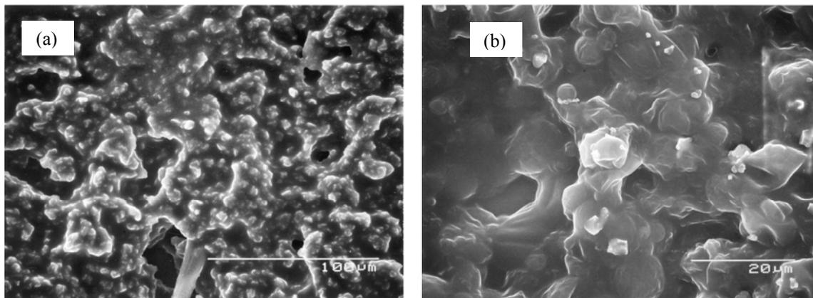
Figure (I)-9. SEM photomicrographs of microcapsules.
