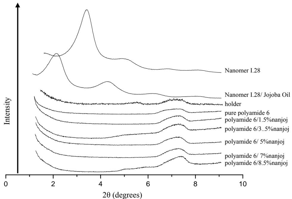
Figure(II)-8: WAXS spectra for pure polyamide 6 and its organoclay-Jojoba Oil nanocomposites with different clay concentrations.
