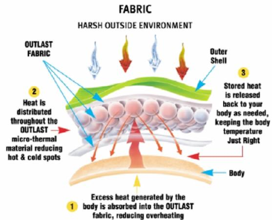
Fig.2: OUTLAST fabric assembling
