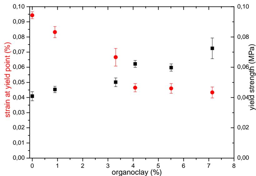
Figure(II)-16: Effect of organoclay content on strain at yield point (●) and yield strength (■) of polyamide 6/organoclay-Jojoba fibers.
