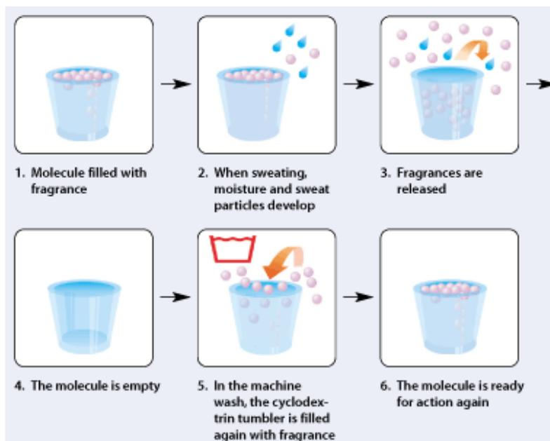
Fig.13: Cyclodextrins action mechanism
