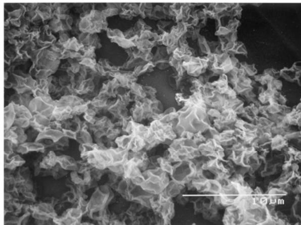
Figure (I)-16. SEM photomicrographs of microcapsules.
