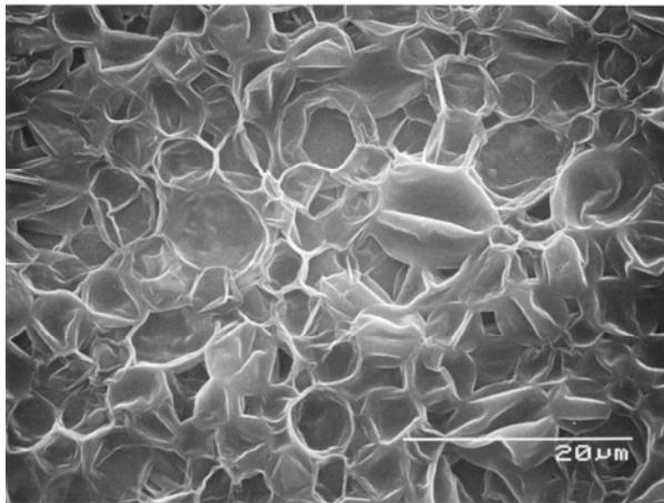
Figure (I)-18. SEM photomicrographs of microcapsules.
