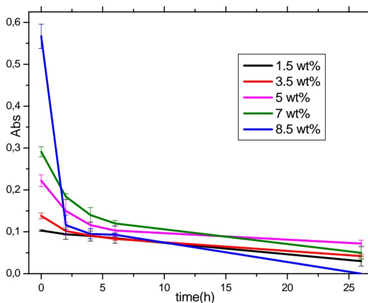
Figure(II)-22: Time release of Jojoba Oil through polyamide 6/organoclay-Jojoba sections
