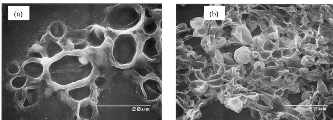
Figure (I)-11. SEM photomicrographs of microcapsules. Effect of cross-linking agent:
