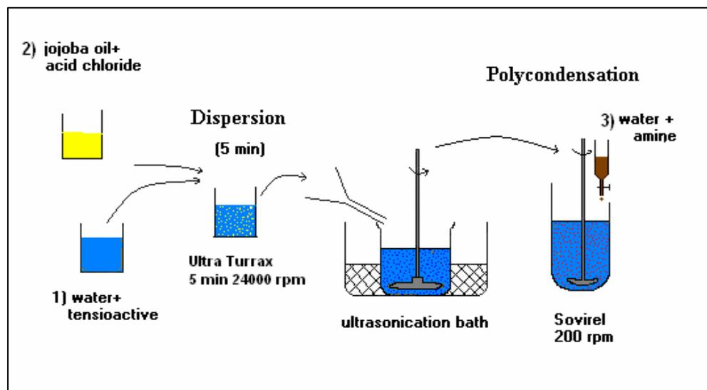
Fig.(I)-8: Three steps of interfacial polymerization reaction
