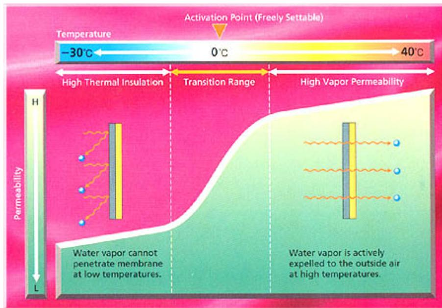
Fig.5: Flexible barrier mechanism with activation point set to 0°C
