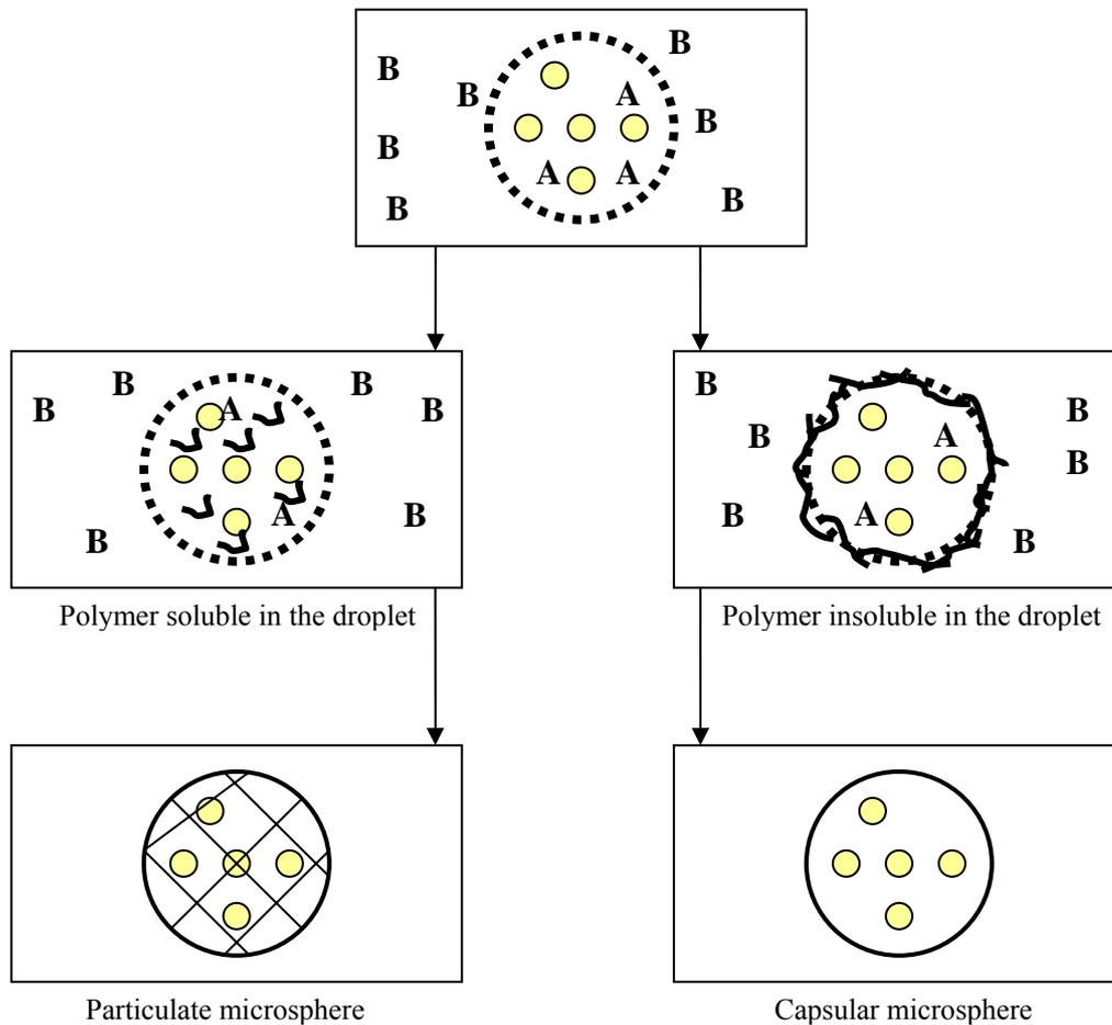
Fig.(I)-4: Idealized mechanism of particle capsule formation by interfacial polycondensation.
