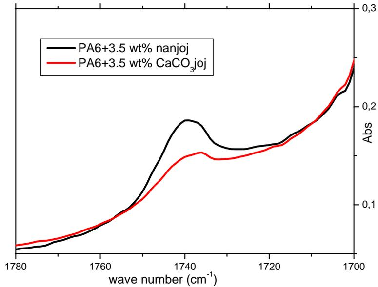
Figure(II)-23: Polyamide 6/organoclay-Jojoba and polyamide 6/ $\text{CaCO}_3$ -Jojoba sections at the same filler content
