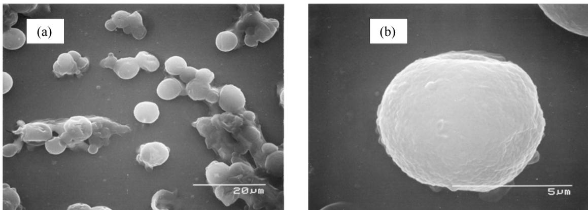
Figure (I)-14. SEM photomicrographs of microcapsules.
