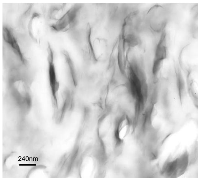
Figure(II)-13: TEM photo of polyamide 6/8.5 wt% nanoj
