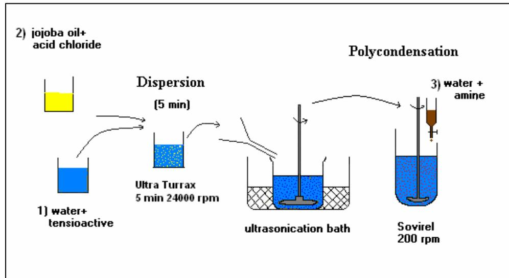
Fig.(I)-8: Three steps of interfacial polymerization reaction
