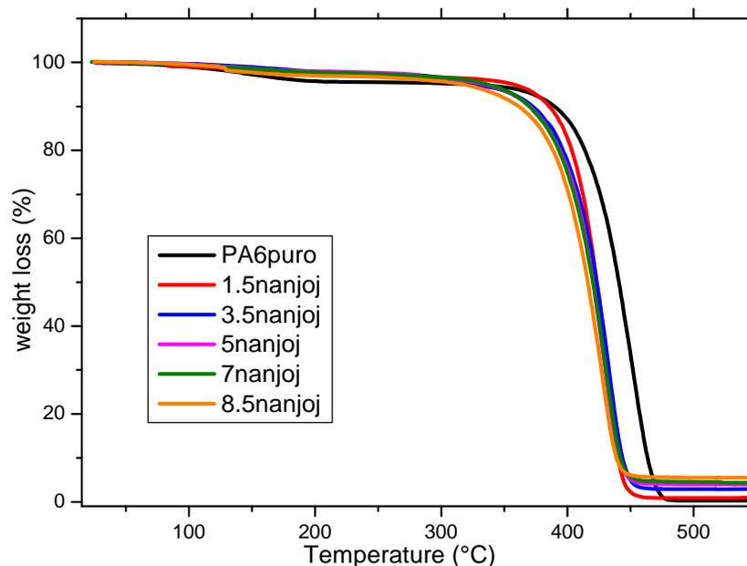
Figure(II)-14: Weight loss as function of temperature of pure polyamide 6 and its nanocomposites.
