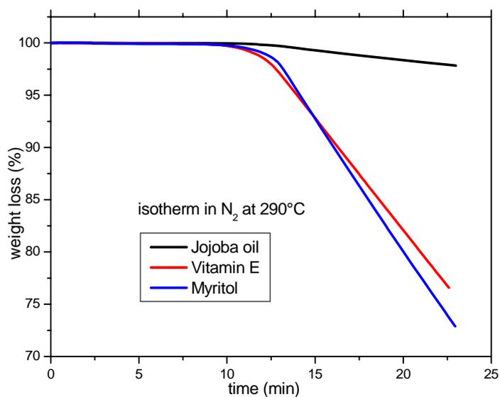
Fig.15: TGA isothermal in N<sub>2</sub>
