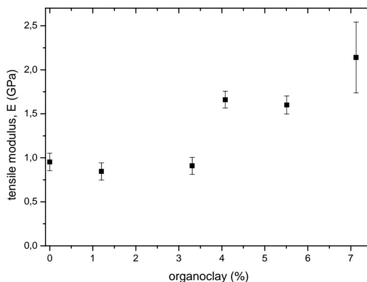
Figure(II)-15:Effect of organolcay content on tensile modulus of polyamide 6/organoclay Jojoba fibers
