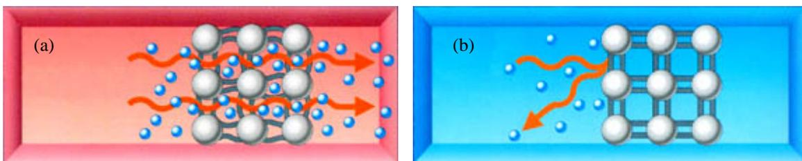
Fig.4: Ambient temperature response function of DiAPLEX fabrics.
