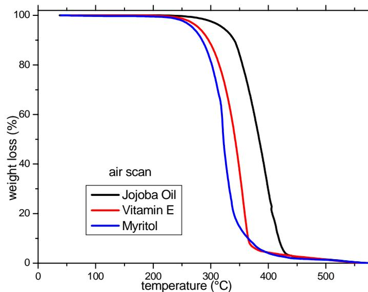
Fig.16: TGA scan in air
