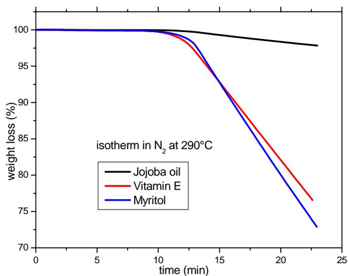
Fig.15: TGA isothermal in N<sub>2</sub>
