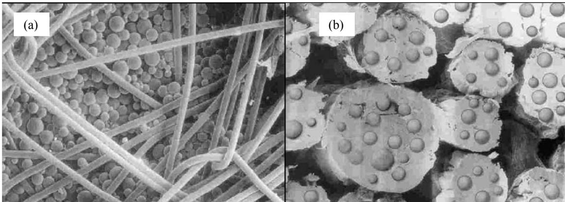
Fig.(I)- 1: (a) PCM microcapsules coated on the surface of fabric and (b) embedded within fibers
