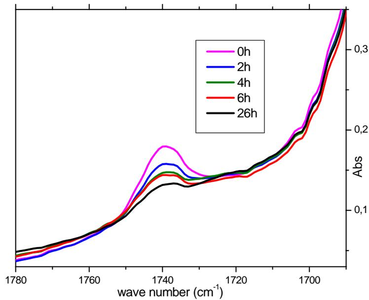
Figure(II)-18: Release of Jojoba Oil through polyamide matrix for polyamide 6/3.5 wt% nanjoj.
