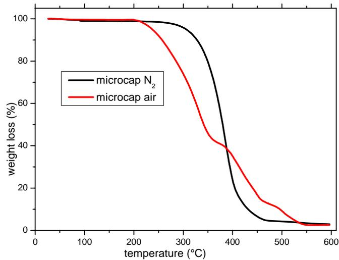
Figure (I)-23. TGA of HMDA/DCT/JOJ microcaps in air and N<sub>2</sub>
