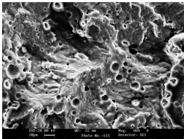
Figure (I)-26. SEM photomicrograph of PA6 matrix containing 10wt% microcapsules
