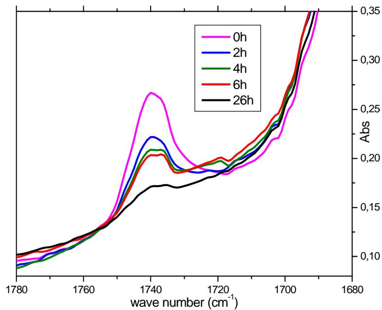
Figure(II)-19: Release of Jojoba Oil through polyamide matrix for polyamide 6/5 wt% nanjoj.
