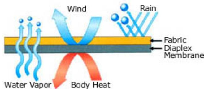
Fig.6: Cross section of DiAPLEX/fabric garment
