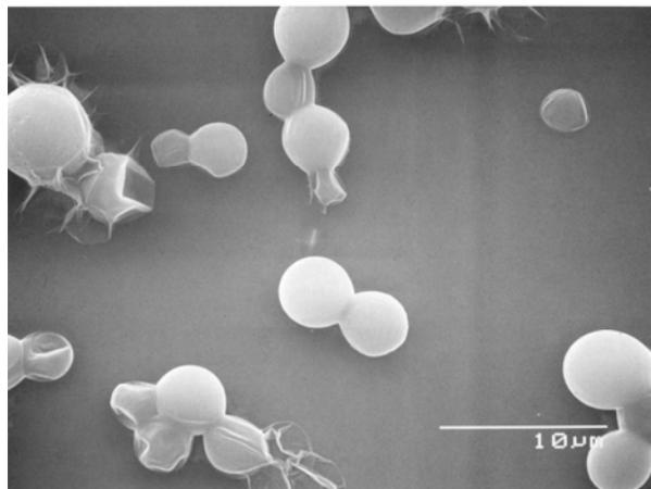
Figure (I)-20. SEM photomicrographs of microcapsules.
