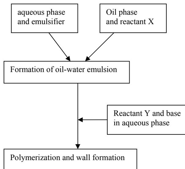
Fig.(I)-3: Scheme of interfacial oil in water polymerization reaction
