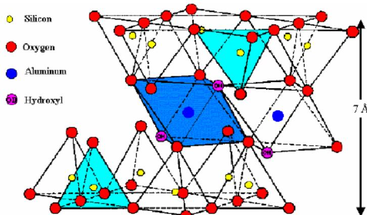
Figure (II)-1: Montmorillonite structure
