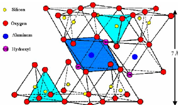
Figure (II)-1: Montmorillonite structure
