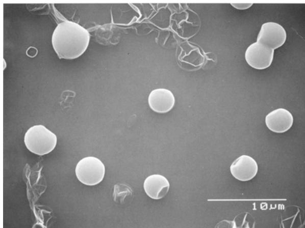
Figure (I)-19. SEM photomicrographs of microcapsules.
