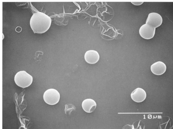
Figure (I)-19. SEM photomicrographs of microcapsules.
