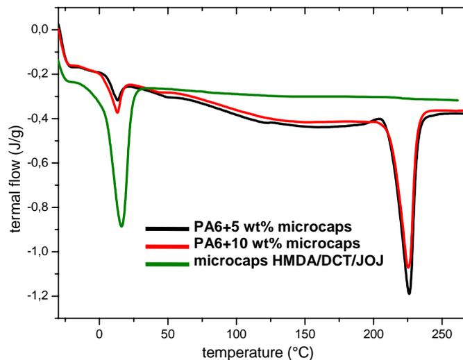
Figure (I)-27. DSC of HMDA/DCT/JOJ microcapsules and PA6 matrix containing 5 and 10 wt% microcapsules
