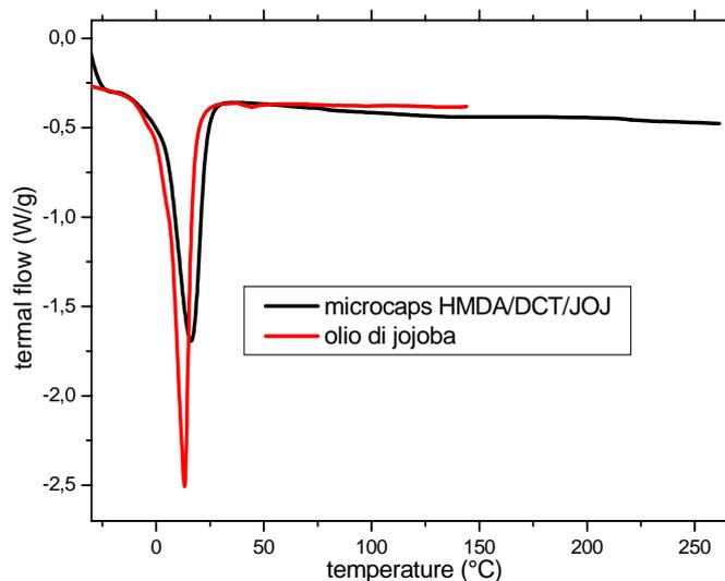
Figure (I)-22. DSC of HMDA/DCT/JOJ microcaps and Jojoba Oil.
