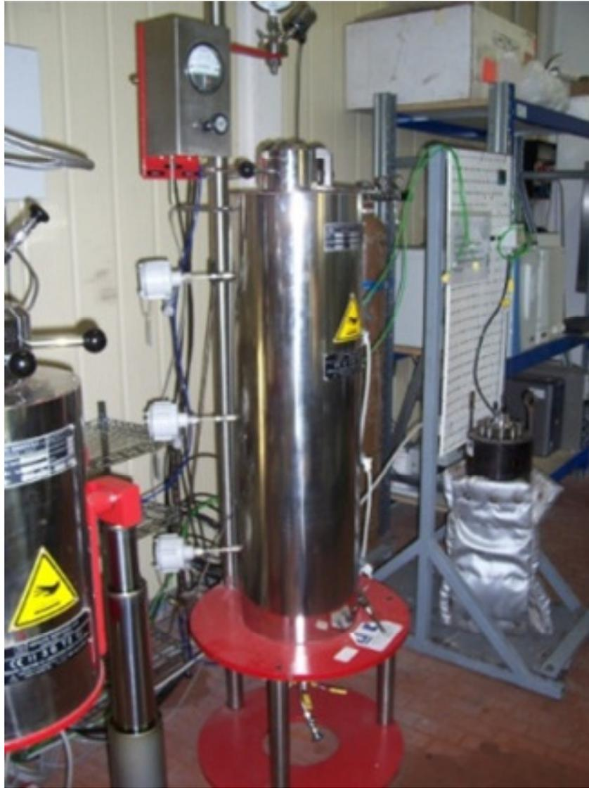
*Figure 13. High pressure tubular vessel*
