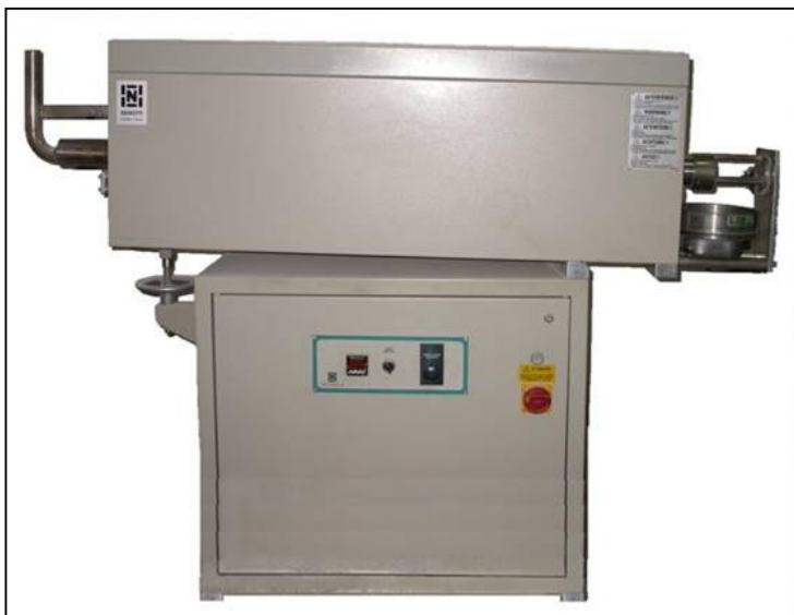
Figure 4. 3: Laboratory rotative kiln (Nannetti mod. TO-R150-15)
