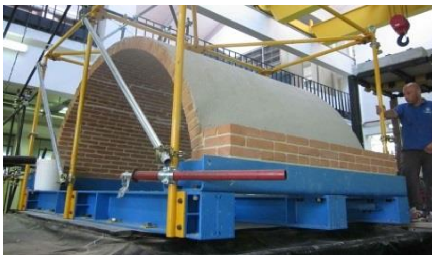
Figure 4.4 IMG system at the extrados of the vault
