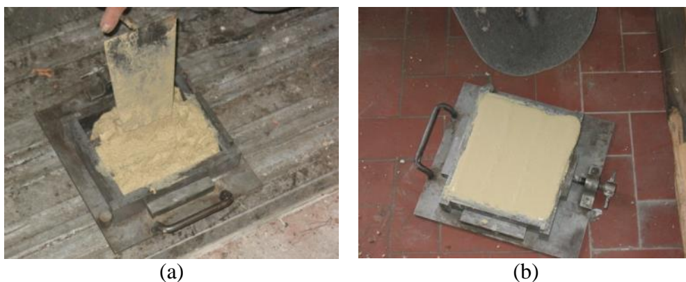
Figure 3.4 Material characterization: mortar specimen preparation
