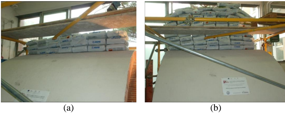
Figure 5.10 Vertical load test: (a) loading phase; (b) maximum load
