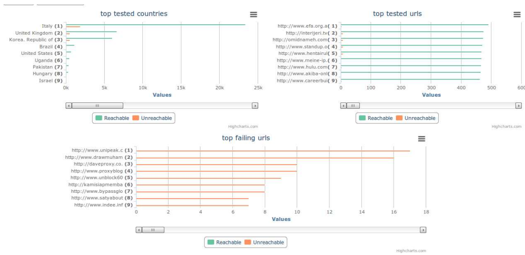
Figure 4.18: UBICA Interface, Global View Reports - middle graphs: bar charts of top tested countries, top tested URLs and top failing URLs (clockwise, from top left). Results are the number of tests for the specific item.
