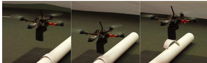
Figure 2.19: images from a sample “swooping” trajectory using the vision-based controller developed in this paper.
