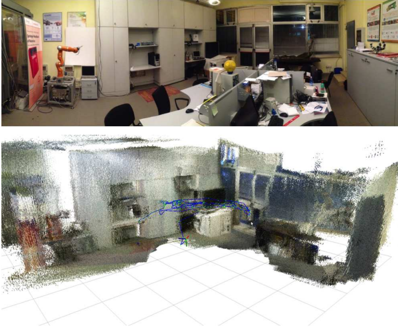
Figure 3.6: Dense colored map reconstruction: on the top the real environment; on the bottom the achieved map. The blue line indicates the sensor motion within the environment as measured by the visual egomotion estimation algorithm with the proposed scale factor computation. The map can be published up to 20 Hz ( F_{max} = 20 Hz and F_{min} = 10 Hz), with \Delta_{R,max} = 10 , \Delta_{R,min} = 5 , \Delta_{C,max} = 20 , \Delta_{C,min} = 10 .
