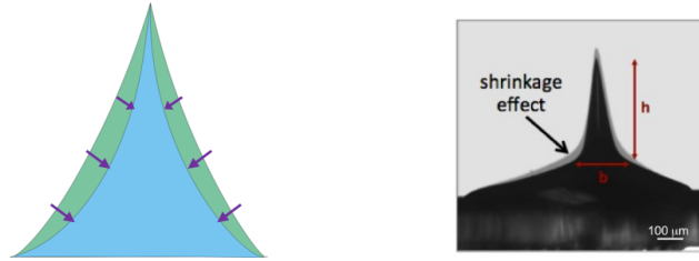
Figure 5.8: Schematic of the thermal treatment and side view of needle before (light gray) and after the thermal treatment.
