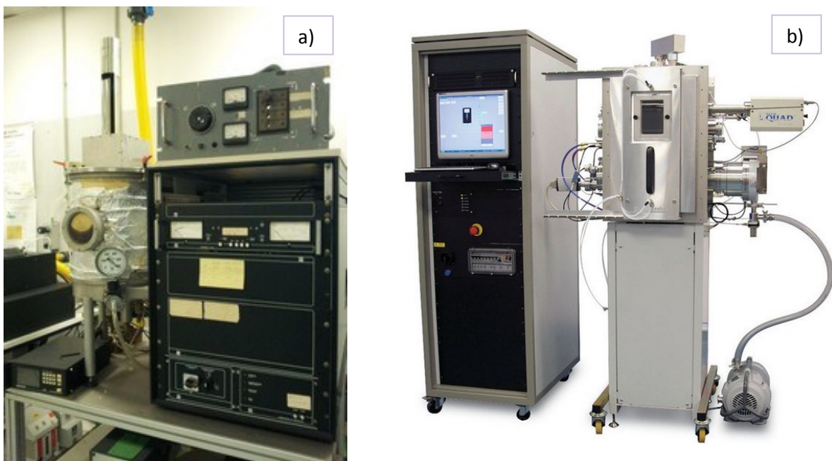
Fig. 6.19: a) Leybold Thermal evaporator @ Cybernetic Institute-CNR (Pozzuoli); b) "Mini-SPECTROS" Thermal evaporator by Kurt J. Lesker Company @ UTTP - ENEA (Portici)
