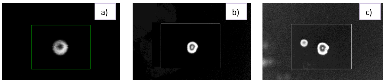
Fig. 6.13: Example of a) lack of focus; b) test made in order to obtain the correct aperture parameter; c) tests made in order to obtain the correct aperture and stigmation parameters
