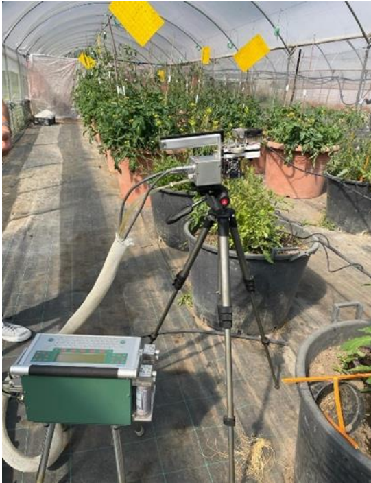
Figure 50. The LI-6400 gas exchange analyzer used in the experiments.
