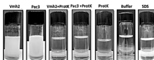
Figure 3. Emulsions between Dectol and protein solutions (0.1 mg/mL, 50 mM TrisHCl pH 8) 2:1 v/v. Starting from the left: emulsions formed by Vmh2, PAC3, and Vmh2 after hydrolysis; PAC3 after hydrolysis; and Proteinase K, buffer, and SDS as controls. Images were acquired after 24 h.
