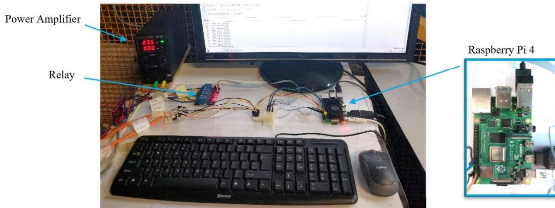
Figure 53. Control circuit for semi-active control.
