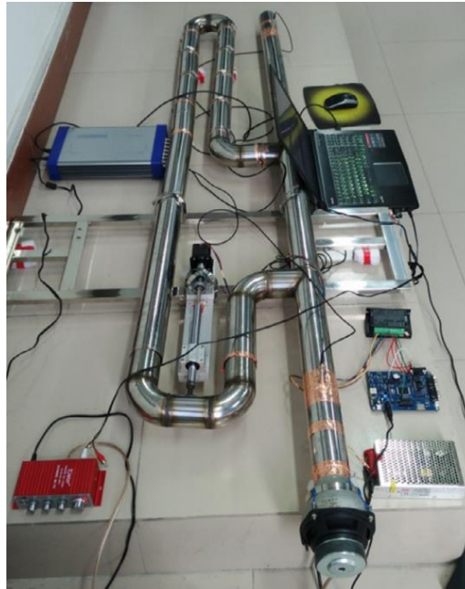
Figure 27. The test stand for semi-active muffler device.
