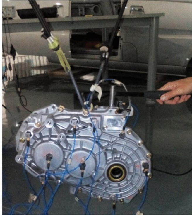
Figure 2. Modal testing of a vehicle gearbox (Zhang, 2018)
