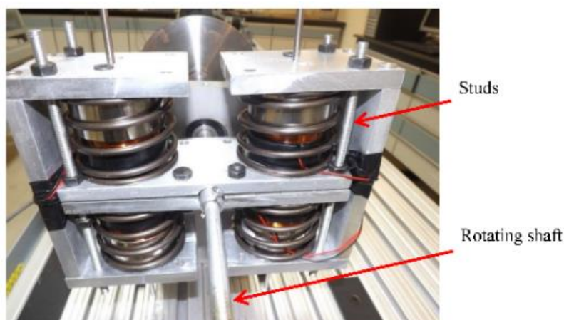
Figure 25 .The adaptive torsional tuned vibration absorber mounted on the rotating shaft.
