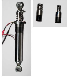
Figure 13. Semi-active actuator (left) with spring components of 163 kN/m and 256 kN/m (right).
