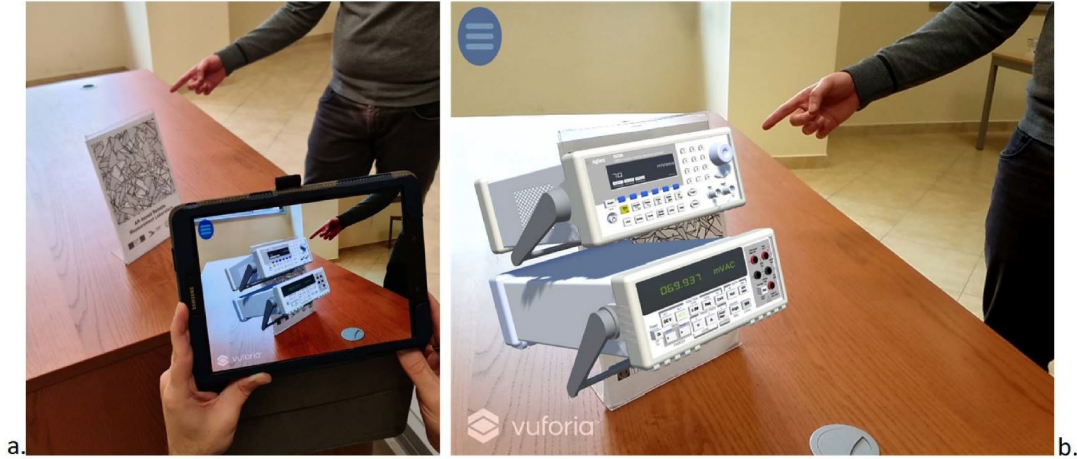
Figure 5. Rendering of the instrumentation due to (a) AR approach and (b) user display screenshot after target identification.
