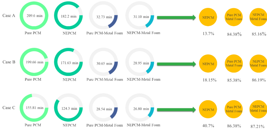
Fig. 3.11. Time-saving in the melting process for all cases with different configurations compared to Case A-pure PCM
