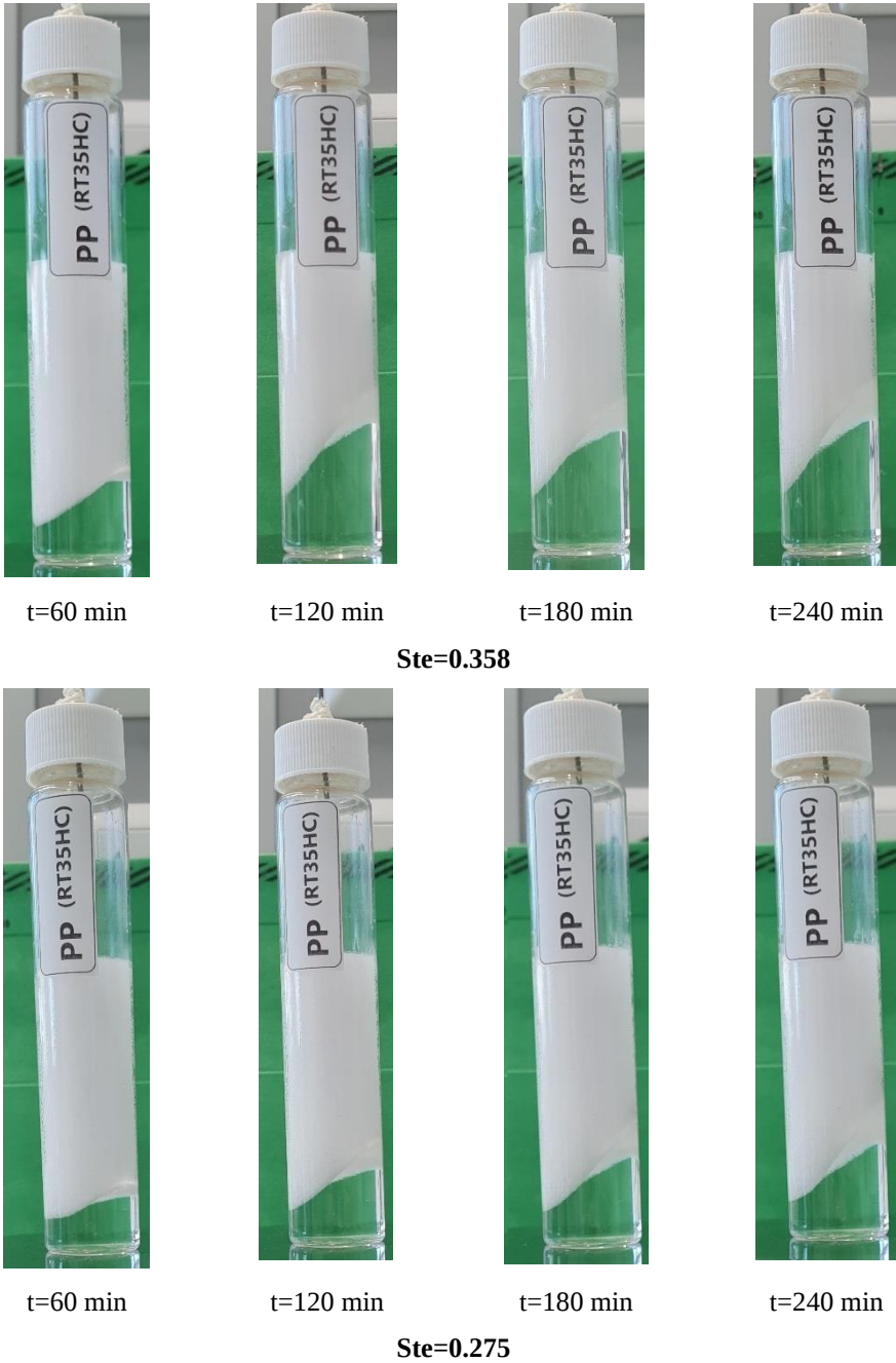
Fig. 5.12 Evolution of melting process of pure PCM (PP) at T_{in}=60^{\circ}\text{C} ( Ste=0.358 ) and T_{in}=50^{\circ}\text{C} ( Ste=0.275 )
