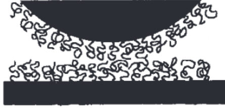
Figure 1.4. Schematic of surface force apparatus experimental setup. End-active polymer chains graft onto crossed mica cylinders and the force between them is measured at various separations. Taken from [15]
