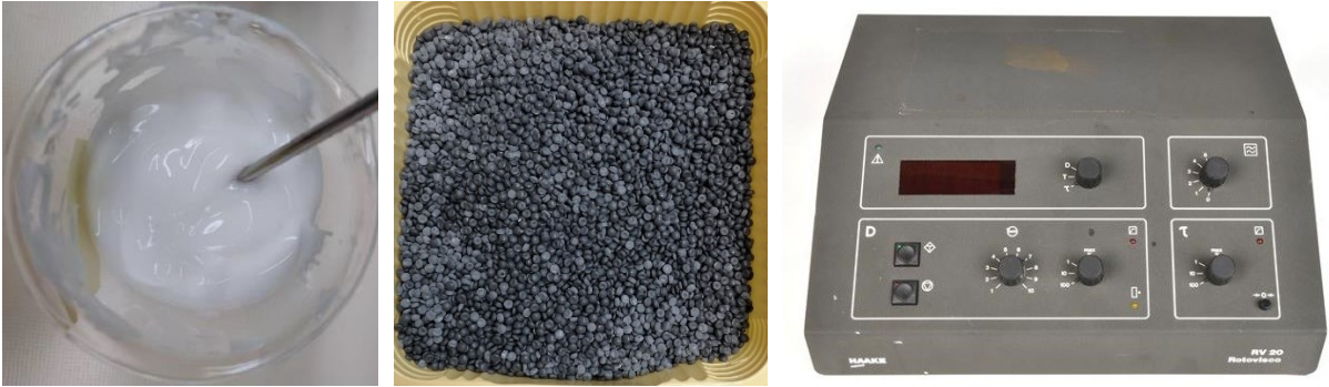
Figure 3. 4. mixture of the viscoplastic shear-thinning fluid (left), LDPE dark-grey particles used as tracers (center), and the Haake Rotovisco RV20-M5 rotational viscometer (right)
