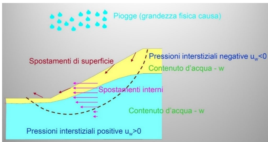
Figure 1.3.1.1: Schematic representation of the physical quantities to be monitored in the case of landslide phenomena. The water content and pore pressures vary in relation to rainfall infiltration and cause both surface and internal slope displacements (Pagano, 2009).
