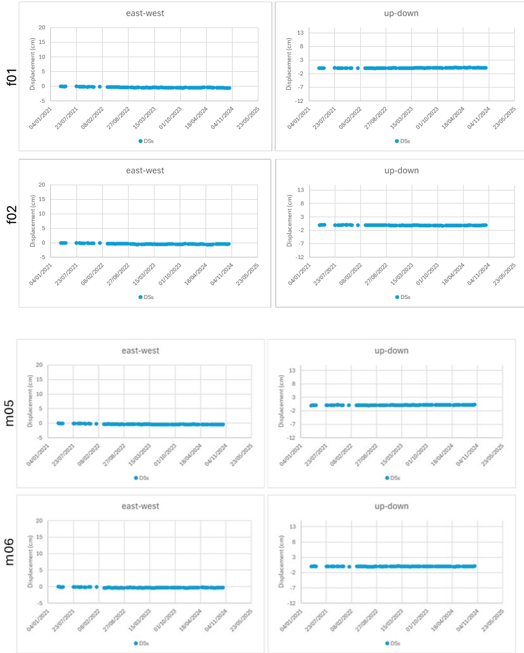
Figure 4.2.7: Time series of the stable Distributed Scatterers (DS), shown in the East–West and vertical (Up–Down) directions. These DS were used for the decomposition of the displacement detected along the satellite Line of Sight (LoS) in both ascending and descending geometries.
