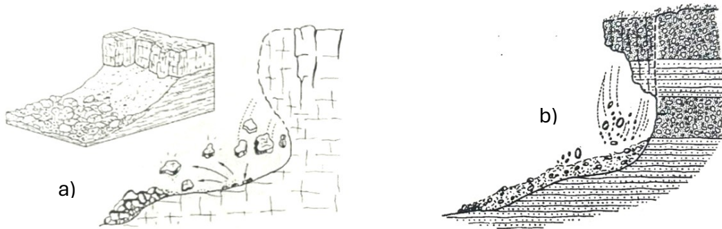
Figure 1.1.5: a) schematic illustration of a rockfall; b) schematic illustration of a fall occurring in poorly consolidated or weathered rocks (Vallario, 1992).
