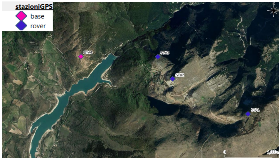
Figure 3.1.4: Map showing the location of the GPS stations. The rovers are depicted in blue, while the base station is shown in magenta.
