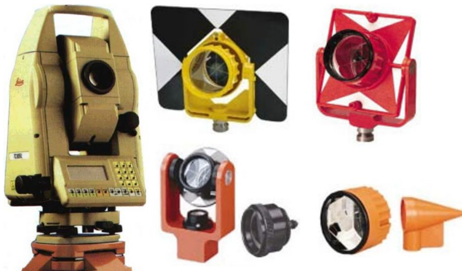
Figure 1.3.3.1: Total station instrumentation and reflective prisms used for topographic measurements.
